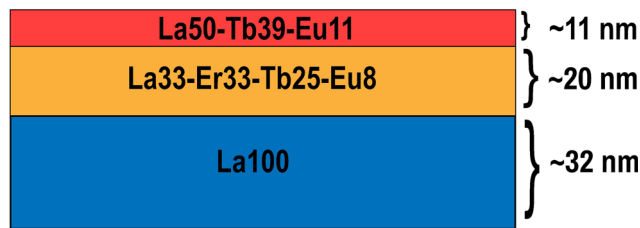
Fig. 4 Schematic illustration of the three-layer composition of the multi-layer La70-Er10-Tb15-Eu5-ML film, of the overall thickness of 63 nm.
