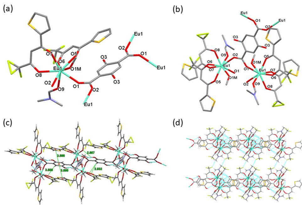
Fig. 2 (a) The asymmetric unit of **Eu2**. (b) Presentation of the dinuclear Eu(III) building blocks in **Eu2**. (c) View of the **Eu2** polymer. (d) View of the 3D supramolecular sheets formed by the **Eu2** CP.
