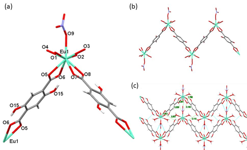
Fig. 1 (a) Presentation of the coordination sphere of Eu(III) in **Eu1**. (b) View of the two-dimensional infinite zig-zag chain formed by **Eu1** CP. (c) View of the 3D supramolecular zigzag sheets formed by **Eu1** CP.
