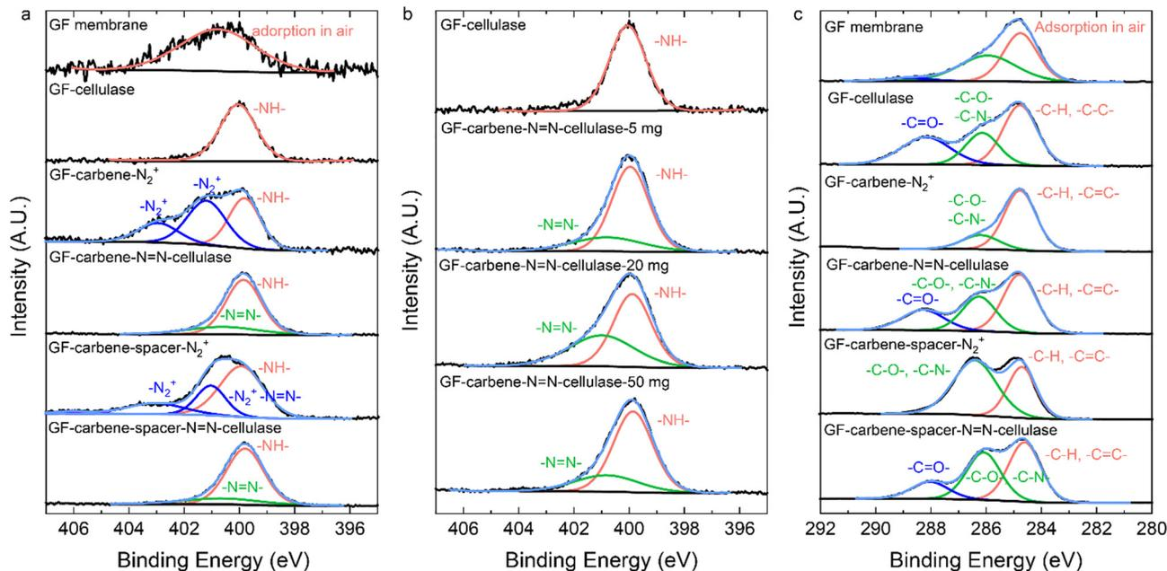
Fig. 3 (a) High resolution N 1s spectra for surfaces of **GF membrane** before and after cellulase immobilization; (b) high resolution N 1s spectra for cellulase on GF modified membrane surface with different  $w$ , where  $w = 0, 5, 20$  and  $50 \text{ mg mL}^{-1}$ ; (c) high resolution C 1s XPS spectra for surfaces of **GF membrane** before and after cellulase immobilization.  $w = 20 \text{ mg mL}^{-1}$  was used to modify **GF membrane**.
