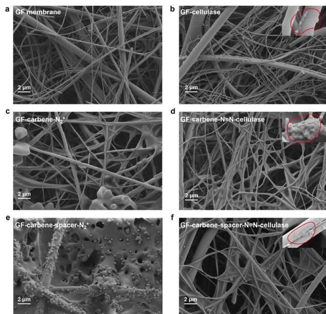
Fig. 5 SEM image for surfaces of (a) **GF membrane**, (b) **GF membrane-cellulase** and insertion at higher magnification, (c) **GF-carbene-N<sub>2</sub><sup>+</sup>**, (d) **GF-carbene-N=N-cellulase** and insertion at higher magnification, (e) **GF-carbene-spacer-N<sub>2</sub><sup>+</sup>**, (f) **GF-carbene-spacer-N=N-cellulase** and insertion at higher magnification. The red circles highlight the aggregated cellulase on the fibers, and  $w = 20 \text{ mg mL}^{-1}$  for the modified membrane.
