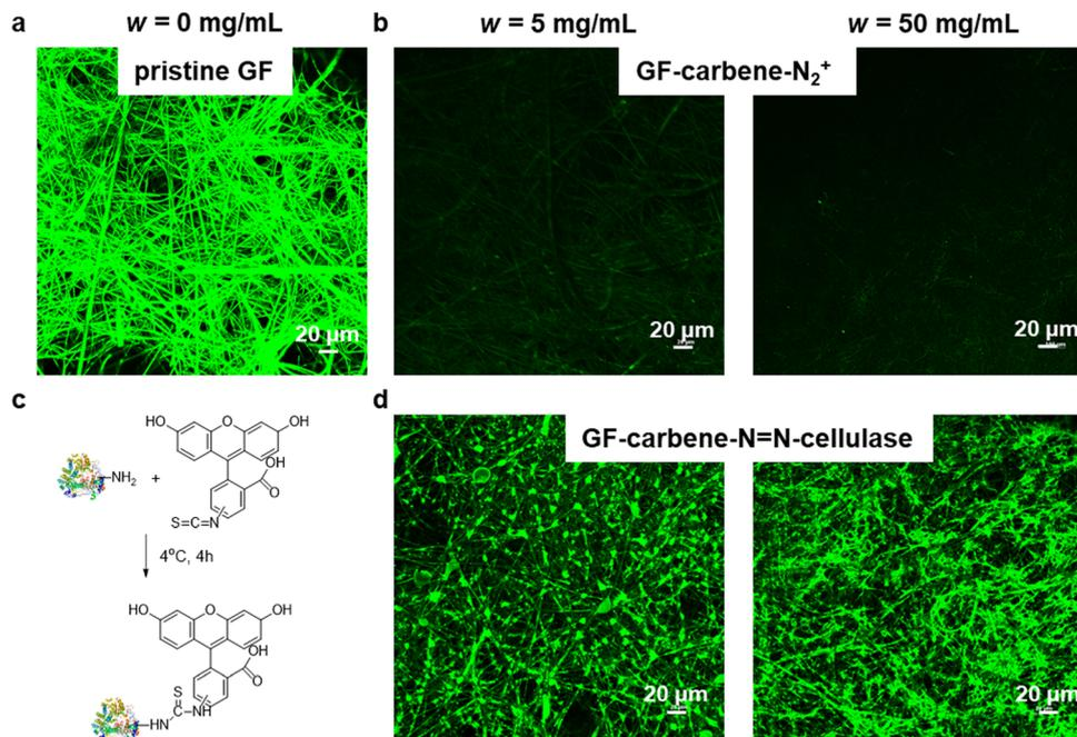
Fig. 6 Visualization of FITC-labelled surface using confocal microscope: (a) pristine GF membrane, (b) GF-carbene-N<sub>2</sub><sup>+</sup> with  $w = 5 \text{ mg mL}^{-1}$  and  $50 \text{ mg mL}^{-1}$ , (c) schematic illustration of FITC with cellulose, (d) GF-carbene-N=N-cellulose with  $w = 5 \text{ mg mL}^{-1}$  and  $50 \text{ mg mL}^{-1}$ .
