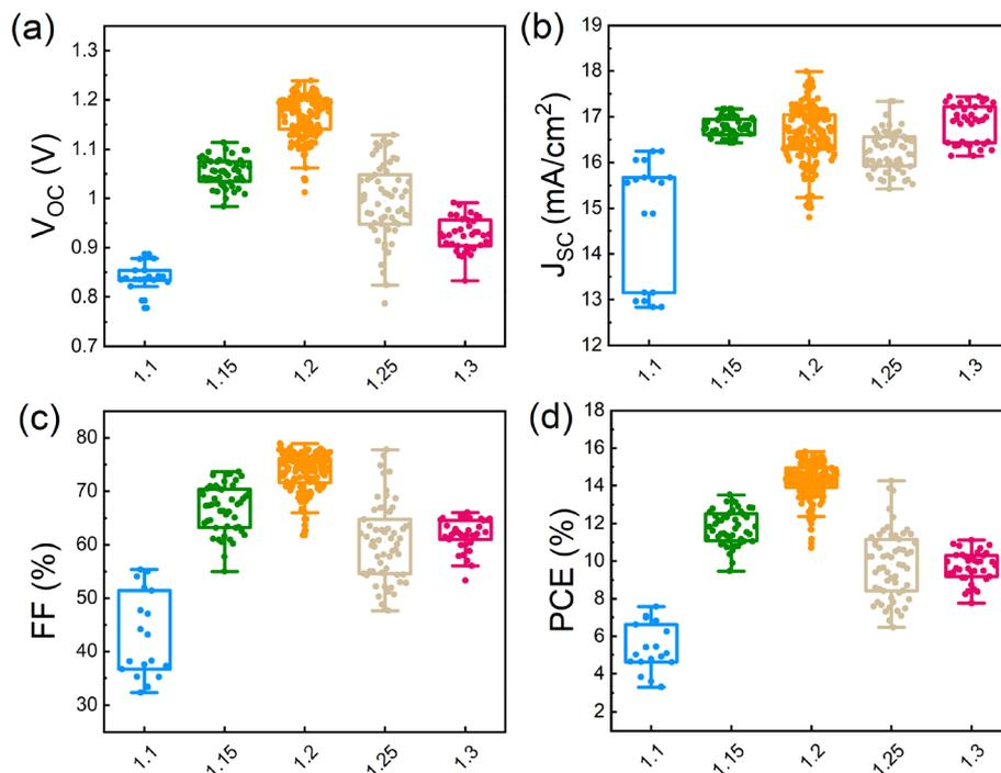
Fig. 5 Photovoltaic performance parameters: (a)  $V_{\text{OC}}$ , (b)  $J_{\text{SC}}$ , (c) FF and (d) PCE distributions of different  $\text{Pb}(\text{OAc})_2$  ratios (1:1, 1:1.5, 1:2, 1:2.5 and 1:3). A total of 350 devices were measured.
