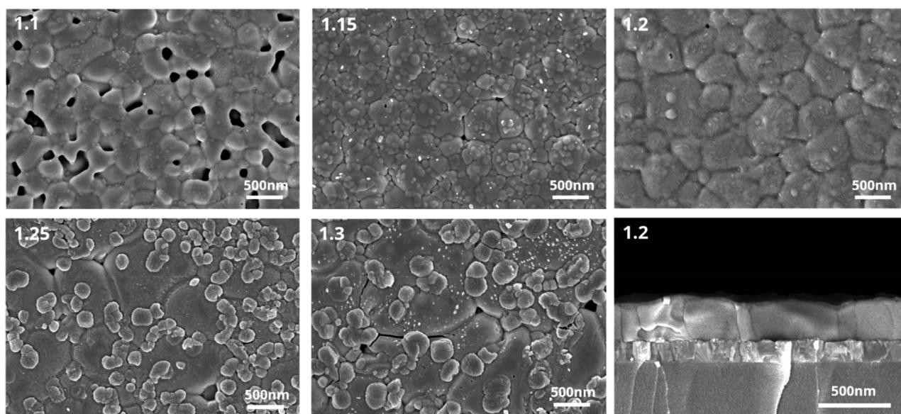
Fig. 3 Scanning electron microscopy images of different  $\text{Pb}(\text{OAc})_2$  ratios ( $X = 1.1, 1.15, 1.2, 1.25$  and  $1.3$ ). Cross-sectional images of 1.2 samples on glass/ITO.
