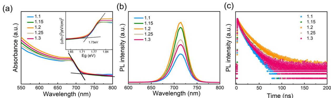
Fig. 4 (a) UV-vis absorbance spectra (inset: Tauc plot for  $\text{CsPbI}_3$  films with different amounts of  $\text{Pb}(\text{OAc})_2$  excess) and (b) steady state and (c) time-resolved photoluminescence emission (PL) spectra of different  $\text{Pb}(\text{OAc})_2$  ratio (1.1, 1.15, 1.2, 1.25 and 1.3) samples.
