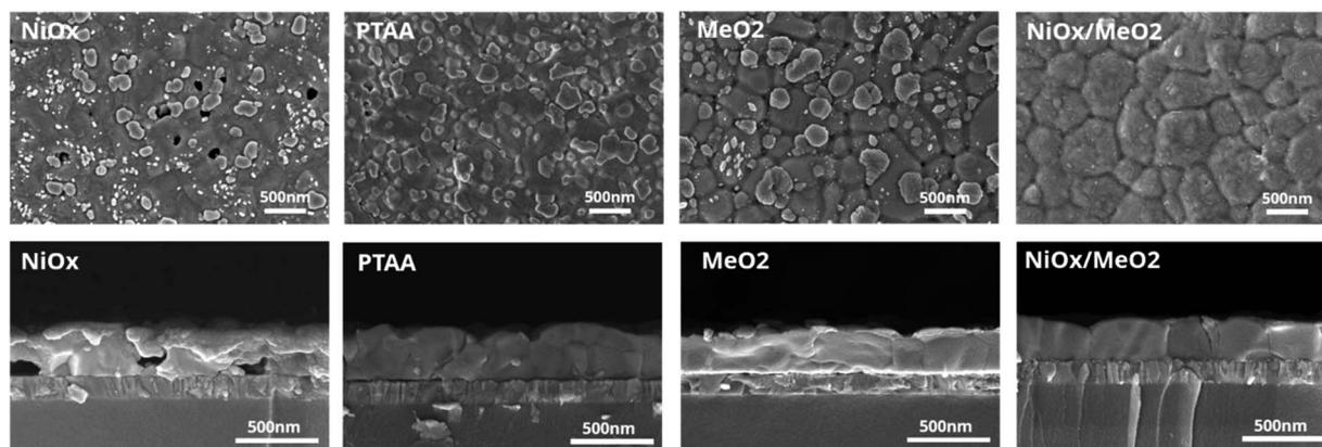
Fig. 6 Top view and cross-section SEM images of  $\text{CsPbI}_3$  films deposited on different hole transport layers ( $\text{NiO}_x$ , PTAA,  $\text{MeO}_2$ , and  $\text{NiO}_x/\text{MeO}_2$ ).
