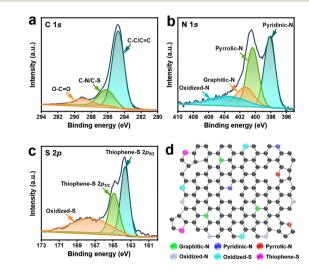
Fig. 3 High-resolution XPS for (a) C 1s, (b) N 1s, and (c) S 2p of NSSC-600. (d) Schematic description of identified bondings of heteroatoms (N and S) in the carbon matrix.
