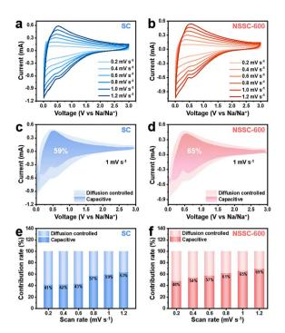
Fig. 6 CV curves of (a) SC and (b) NSSC-600 at the scan rates from 0.2 to 1.2 mV s<sup>-1</sup>. Capacitive contribution area of (c) SC and (d) NSSC-600 at 1.0 mV s $^{-1}$ . Capacitive contribution ratios of (e) SC and (f) NSSC-600 at the scan rates from 0.2 to 1.2 mV s<sup>-1</sup>
