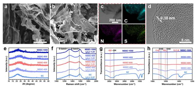
Fig. 2 FESEM image of (a) SC and (b) NSSC-600. (c) Elemental mapping for C, N, and S and (d) HRTEM images of NSSC-600. (e) XRD, (f) Raman spectra and (g and h) FTIR spectra of SC, NSSC-400, NSSC-600, NSSC, and NSSC-1000. Note: as the carbon precursor is derived from the natural sugarcane biomass, potential impurities were identified in the XRD spectra.
