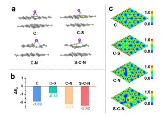
Fig. 5 DFT calculations: (a) the calculation models, (b) the adsorption energy, and (c) the electronic localization function of C, C–S, C–N, and S–C–N after K adsorption. The grey, yellow, cyan and violet balls indicate the C, S, N, and K atoms, respectively.
