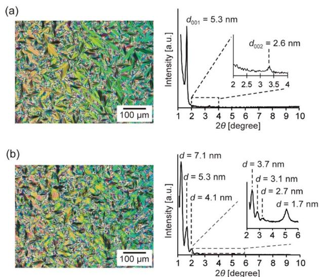
Fig. 4 POM images and XRD patterns of compound **1** and polymerized **1** (**P1**) in their SmA phases. (a) POM image (left) and XRD pattern (right) of compound **1** at 100 °C. (b) POM image (left) and XRD pattern (right) of **P1** at 100 °C.
