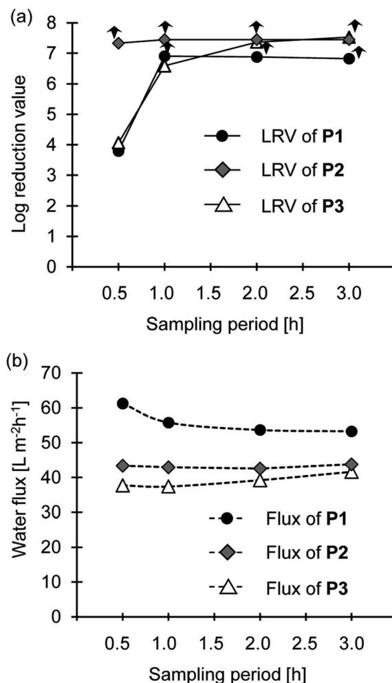
Fig. 6 Performance of **P1**, **P2** and **P3** membranes as virus filtration membranes. (a) Log reduction value (LRV) for Q $\beta$  and (b) water flux through **P1**, **P2** and **P3** membranes. Arrows indicate right-censoring LRVs.
