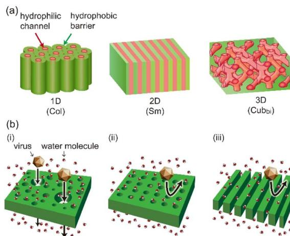
Fig. 1 (a) Schematic illustration of liquid-crystalline (LC) nanopores. Self-organized columnar (Col), smectic (Sm) and bicontinuous cubic ( $Cub_{bi}$ ) phases form one-, two- and three-dimensional (1D, 2D and 3D) nanochannels, respectively. (b) Schematic illustration of virus rejection by various porous membranes: (i) conventional membrane with pore-size distribution, (ii) nano-ordered membrane and (iii) smectic membrane with 2D pores.
