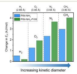
Fig. 8 Comparison of changes in activation energy of permeation  $(E_{\rm p})$  for PIM-NH $_2$  and PIM-NH $_2$ -FVM samples upon aging. The samples were aged for 710 h.
