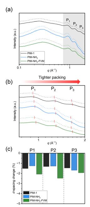
Fig. 9 Comparison of wide-angle X-ray scattering patterns on a (a) full scale and (b) magnified scale for PIM-1, PIM-NH<sub>2</sub>, and PIM-NH<sub>2</sub>-FVM. The fresh samples are represented by dotted lines, while the samples that have been aged for approximately 1400 h are represented by solid lines. The red dotted lines in (b) represent the peak values used to calculate the d-spacing, and the changes in the d-spacing obtained from the patterns are shown in (c).
