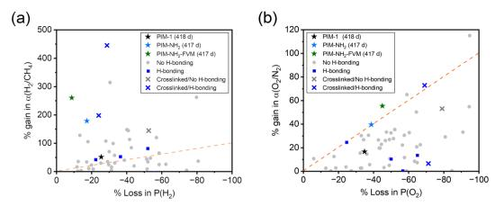
Fig. 5 Comparison of long-term physical aging effects on (a)  $H_2/CH_4$  and (b)  $O_2/N_2$  separation for various PIMs reported in the literature. The star symbols are PIMs in this study, and only polymer films with a minimum of 100 days of aging are considered. The dotted orange line is a parity line, representing equal permeability loss and selectivity gain.
