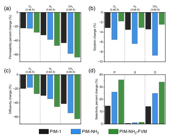
Fig. 6 Percent changes in (a) permeability, (b) sorption, (c) diffusivity, and (d) O<sub>2</sub>/N<sub>2</sub> selectivities over approximately 2230 h of physical aging. The gases are ordered from smallest to largest kinetic diameters, and gray dashed lines separate the three tested gases (O2, N2, and CH4) in figures a-c.
