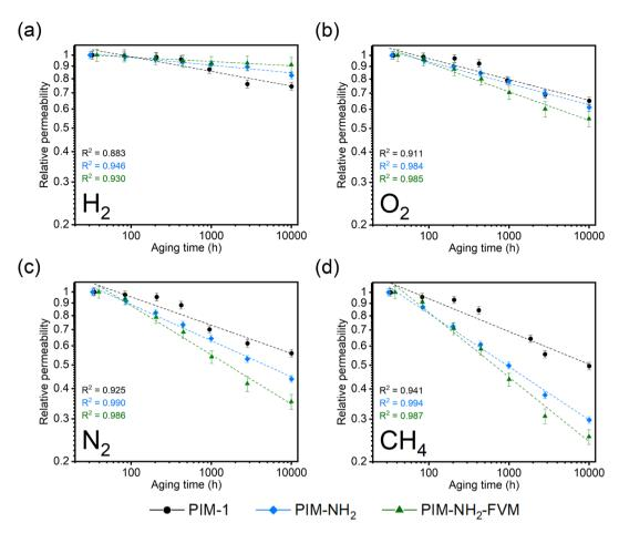
Fig. 2 Comparison of aging behavior by tracking pure-gas permeabilities on a normalized scale for (a)  $H_2$ , (b)  $O_2$ , (c)  $N_2$ , and (d)  $CH_4$ . All data have been normalized to the first data point to show relative permeability. The linear fits of the experimental data on a log-log scale are shown in the dashed lines along with their  $R^2$  values.
