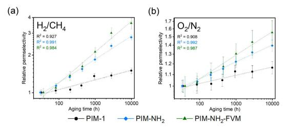
Fig. 4 Comparison of selectivity as a function of time on a normalized scale for (a)  $H_2/CH_4$  and (b)  $O_2/N_2$ . All data have been normalized to the first data point to show relative selectivity. The linear fits of the experimental data on a log-log scale are shown in the dashed lines along with their  $R^2$  values.
