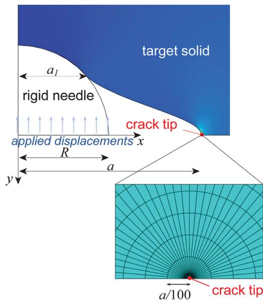
Fig. 7 Deformed configuration of the FE model under full penetration of the needle, with relative radius  $R/a = 0.5$ , being  $a$  the initial crack length in the undeformed solid. Inset shows a detail of the mesh adopted in the crack tip region. Note that the crack length  $a$  and the contact length  $a_1$  depicted in the figure refer to the deformed configuration of the target solid.
