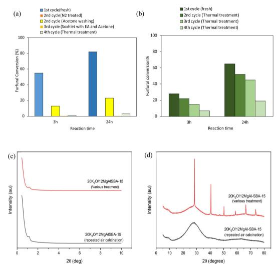
Fig. 5 Reusability performance of the re-used 20K<sub>2</sub>O/12MgAl-SBA-15 over four reaction cycles with (a) four different treatments, including calcination under a N<sub>2</sub> environment, acetone washing and drying, cleaning with Soxhlet apparatus using ethyl acetate (EA), followed by acetone washing and open-air calcination, and (b) four consecutive open-air calcinations; (c) low-angle, and (d) wide angle XRD of the calcined catalysts regenerated after the fourth cycle.
