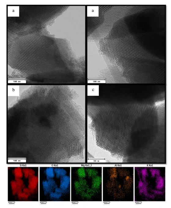
Fig. 2 TEM images for (a) SBA-15 (b) 12-MgAl-SBA-15 and (c) 20K<sub>2</sub>O/12MgAl-SBA-15 and elemental mapping of 20K<sub>2</sub>O/12MgAl-SBA-15.
