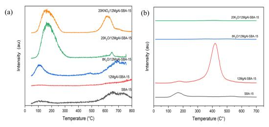
Fig. 3 (a) CO<sub>2</sub>-TPD and (b) TGA-MS-propylamine of parent and modified SBA-15
