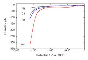
Fig. 2 LSVs using the complex-modified glassy carbon electrode in a 0.10 M phosphate buffer solution (pH 7.0). Working electrode: glassy carbon (0.071 cm $^2$ ) modified with Co<sub>2</sub>DNCH and MW-CNT (a), CoPF<sub>5</sub> and MW-CNT (b), MW-CNT (c), bare glassy carbon (d), counter electrode: Pt wire, reference electrode: SCE, scan rate: 0.10 V s $^{-1}$ , temp: 295 K.
