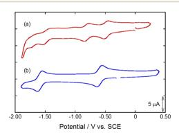
Fig. 3 CVs of DMF solutions containing  $Co_2DNCH$  (a) and  $CoPF_5$  (b). Working electrode: glassy carbon (0.071 cm<sup>2</sup>), counter electrode: Pt, reference electrode: Ag/AgNO<sub>3</sub>, complex: 0.25 mM, electrolyte: n-Bu<sub>4</sub>NClO<sub>4</sub> (100 mM), scan rate: 0.10 V s<sup>-1</sup>, temp: 295 K. All potentials were converted to voltages vs. SCE.
