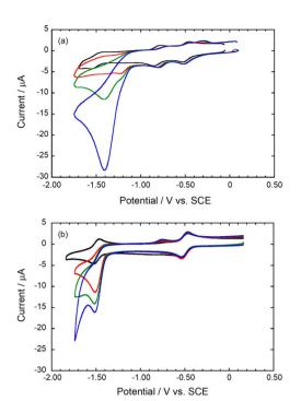
Fig. 5 CVs of the DMF solutions of  $Co_2DNCH$  (a) and  $CoPF_5$  (b) in the absence (black) and presence of triethylammonium chloride: 2.0 (red), 5.0 (green) and 10 equiv. (blue). Working electrode: glassy carbon (0.071 cm²), counter electrode: Pt, reference electrode: Ag/AgNO<sub>3</sub>, complex: 0.25 mM, electrolyte: n-Bu<sub>4</sub>NClO<sub>4</sub> (100 mM), scan rate: 0.10 V s<sup>-1</sup>, temp: 295 K. All potentials were converted to voltages vs. SCE.
