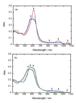
Fig. 4 UV-vis absorption spectra of the DMF solutions of Co<sub>2</sub>DNCH (0.14 mM) before (red in (a)) and after controlled-potential electrolysis at -0.6 V (blue in (a) and (b)) and -1.0 V (green in (c)). Optical path length: 0.5 mm, working electrode: Pt mesh, counter electrode: Pt wire, reference electrode: Aq/AqNO<sub>3</sub>, electrolyte: n-Bu<sub>4</sub>NClO<sub>4</sub> (100 mM). All potentials were converted to voltages vs. SCE.
