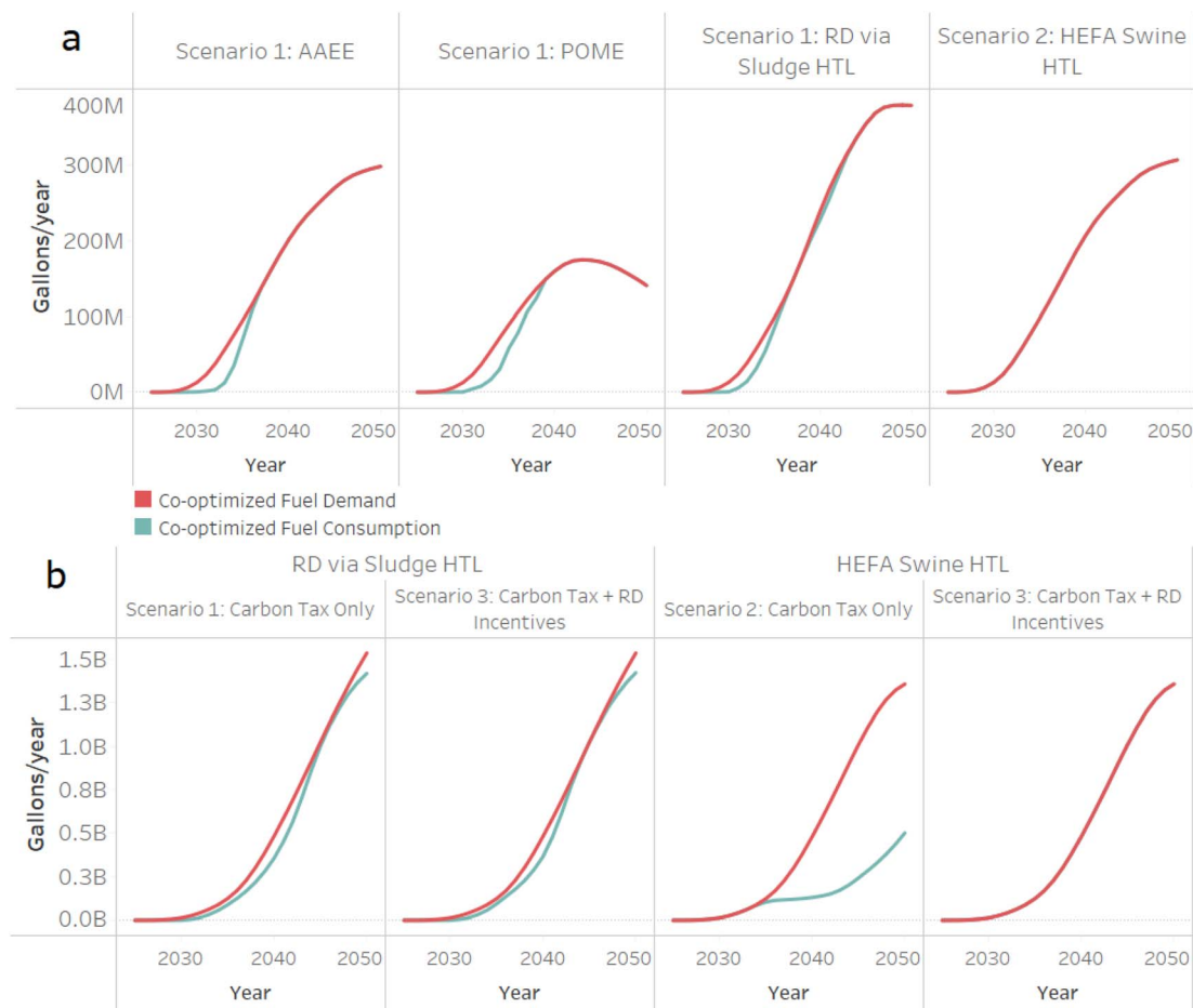
Fig. 4 Co-optimized fuel demand versus consumption (gallons per year) by co-optimized vehicles in the no carbon tax case (panel a) and in the carbon tax case, with and without additional renewable diesel incentives (panel b), 2020–2050. Note that HEFA swine HTL refers to HEFA transitioning to HTL.
