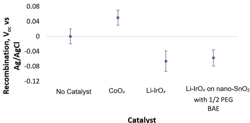
Fig. 3  $V_{oc}$  vs. Ag/AgCl reference electrode in a half-cell setup for nano-SnO<sub>x</sub>C<sub>y</sub>/PMPDI anodes with differing catalyst addition. Note, no catalyst is added to the far-left data point. In this system,  $V_{oc} \approx E_{F,n}$ , the quasi-Fermi energy of electrons in the SnO<sub>2</sub> sub-bandgap states.<sup>12,13</sup>
