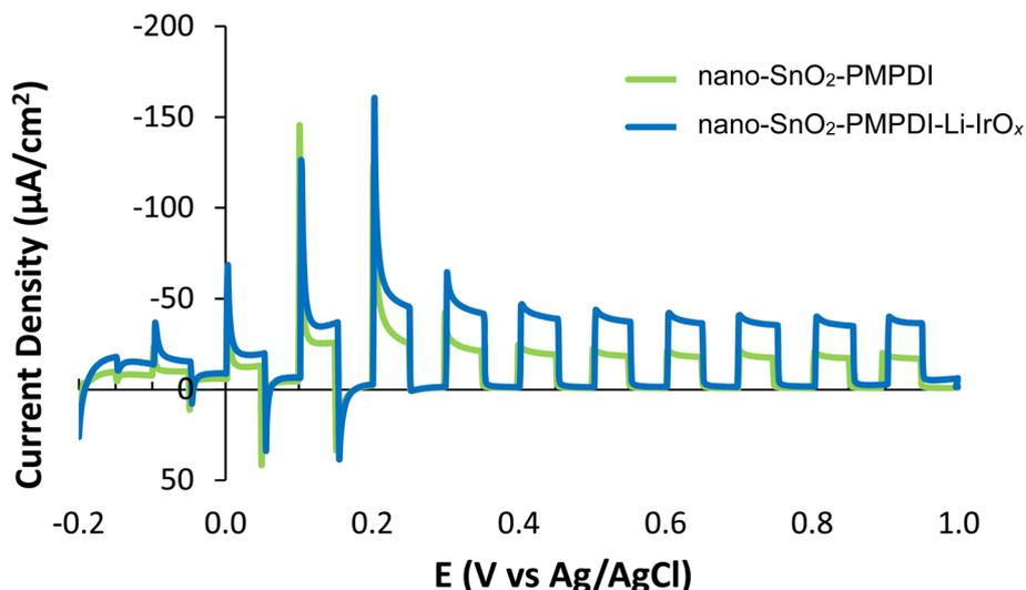
Fig. 2 Photocurrent transients for nano-SnO<sub>x</sub>C<sub>y</sub>/PMPDI (green) and nano-SnO<sub>x</sub>C<sub>y</sub>/PMPDI/Li-IrO<sub>x</sub> (blue) anodes in pH 7, 0.1 M KPi buffer. Scans were done from -0.2 to +1.0 V vs. Ag/AgCl with 5 s light dark transients.
