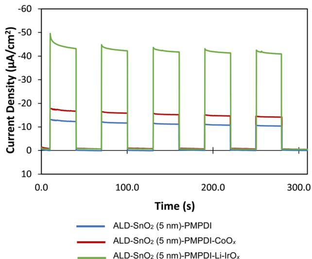
Fig. 7  $J-t$  transients in the presence of 20 mM  $H_2Q$  sacrificial reductant, with background dark current subtracted, at +0.2 V vs. Ag/AgCl in pH 7, 0.1 M KPi buffer with 30 s light/dark transients where blue is ALD- $SnO_2(5\text{ nm})/PMPDI$ , red is ALD- $SnO_2(5\text{ nm})/PMPDI/CoO_x$ , and green is ALD- $SnO_2(5\text{ nm})/PMPDI/Li-IrO_x$  (green) anodes.
