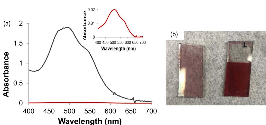
Fig. 4 (a) Optical absorbance spectrum of PMPDI on  $\text{SnO}_x\text{C}_y$  (black) and PMPDI on ALD- $\text{SnO}_2$  (red). Absorbance of bare  $\text{SnO}_2$  film was subtracted off. The insert shows a zoomed-in plot of the absorbance of PMPDI on ALD- $\text{SnO}_2$ . (b) Image of ALD- $\text{SnO}_2$ /PMPDI anode (left) and nano- $\text{SnO}_x\text{C}_y$ /PMPDI anode (right), where only the bottom two thirds of the anode is dyed.
