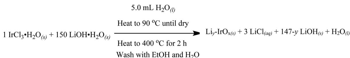
Scheme 1 Literature-based synthesis of Li-IrO<sub>x</sub> following Gao and coworkers experimental.<sup>35</sup>
