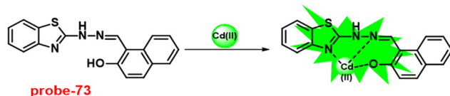
Fig. 107 Chemical structure and proposed sensing mechanism of probe-73 with Cd(II) (redrawn the ChemDraw structure from ref. 63).
