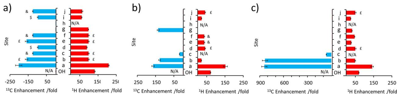
Fig. 3 Comparison of  $^1\text{H}$  and  $^{13}\text{C}$  NMR signal enhancements for (a) **1** (b) **2** and (c) **3** when a sample of each (25 mM) is shaken with  $[\text{IrCl}(\text{COD})(\text{IMes})]$  (5 mM),  $\text{NH}_3$  (25 mM) and  $p\text{-H}_2$  (3 bar) in  $\text{DCM-}d_2$  (0.6 mL) for 10 seconds at 6.5 mT. Note that the symbols £, \$ and & indicate signal overlap and therefore the signal enhancement quoted reflects an average of the two sites.
