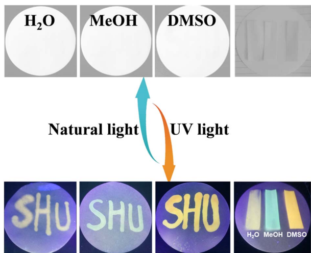
Fig. 7 The photos of the \text{Vio1}\cdot\text{2Cl} dispersed test papers after treatment with different organic solvents under natural light and UV light.
