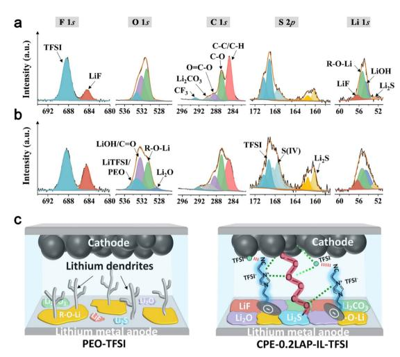
Fig. 5 High-resolution spectra of F 1s, O 1s, C 1s, S 2p, and Li 1s for Li electrodes dissembled from (a) Li||PEO-TFSI||Li and (b) Li||CPE-0.2LAP-IL-TFSI||Li cells after cycling at 0.1 mA cm<sup>-2</sup> for 50 h; (c) schematic illustration of lithium dendrites formation, chemical components on lithium metal anode and Li<sup>+</sup> transference pathway within ASSLMBs with PEO-TFSI or CPE-0.2LAP-IL-TFSI membranes.
