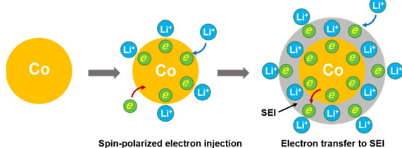
Fig. 4 Schematic illustrations of lithium storage in metallic Co via a spin-polarized electron injection to the 3d orbital of Co and subsequent electron transfer to the surrounding SEI at lower potential.
