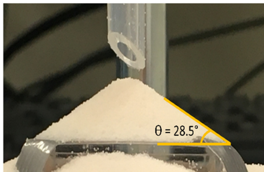
Fig. 2 Image resulting from the angle of repose tests of the alumina particles.
