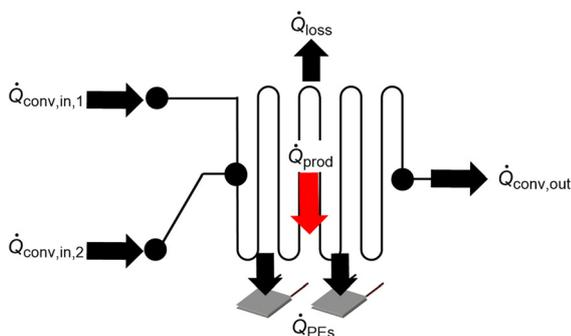
Fig. 5 Schematic representation of the system's energy balance.
