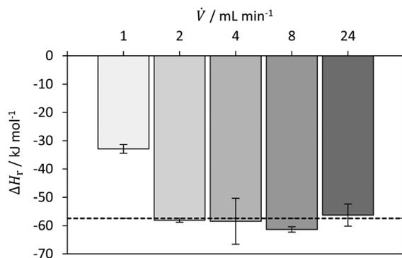
Fig. 7 Determined reaction enthalpy for neutralization of HCl with NaOH in isoperibolic operation mode with comparison to literature value (dashed line) from Riedel and Meyer<sup>50</sup> (2018).
