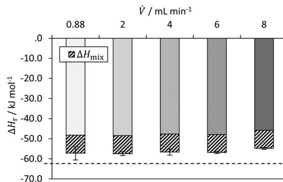
Fig. 11 Determined reaction enthalpy for hydrolysis of acetic anhydride in isothermal operation mode with comparison to literature value (dashed line) from Ładosz *et al.*<sup>25</sup> (2020).
