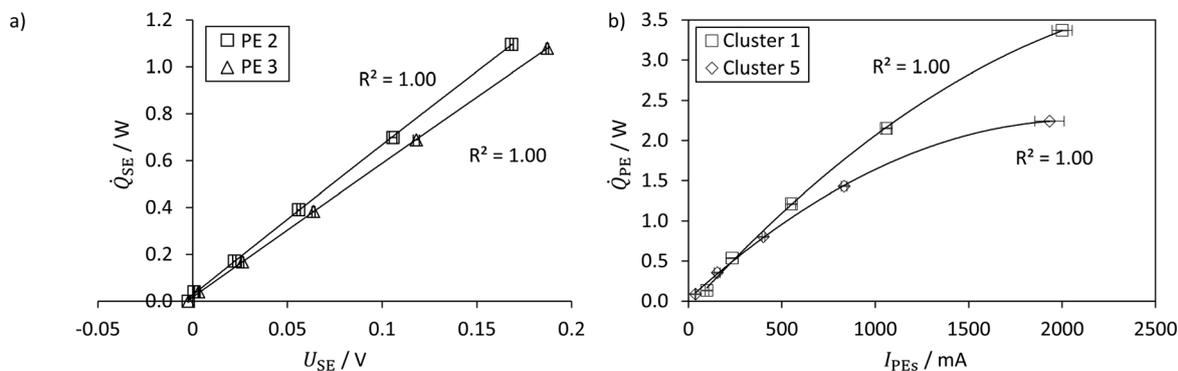
Fig. 6 a) Direct correlation of applied heat flux and measured thermoelectric voltage of two PE2 and PE3 for  $T_{\text{MB}} = 25 \text{ }^\circ\text{C}$ . b) Direct correlation of dissipated heat flux and supplied electrical current of cluster 1 and 5 for  $T_{\text{MB}} = 30 \text{ }^\circ\text{C}$ .
