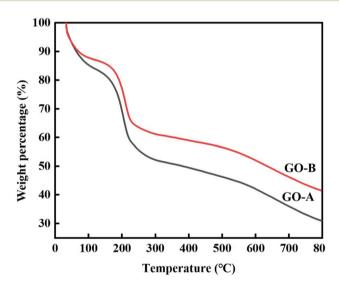
Fig. 6 TGA curves of the GO-A and GO-B.
