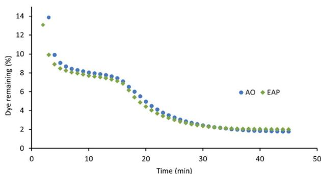
Fig. 11 AO- and EAP-mediated decolorisation of Acid Red 87 as a function of time. AO conditions:  $[\text{AR87}] = 100 \mu\text{M}$ , graphite anode and cathode,  $[\text{Na}_2\text{S}_2\text{O}_8] = 14 \text{ mM}$ ,  $I = 5 \text{ mA}$ , stirring = 1000 rpm. EAP conditions:  $[\text{AR87}] = 100 \mu\text{M}$ , boron-doped diamond anode, graphite cathode,  $[\text{Na}_2\text{S}_2\text{O}_8] = 14 \text{ mM}$ ,  $I = 5 \text{ mA}$ , stirring = 1000 rpm.
