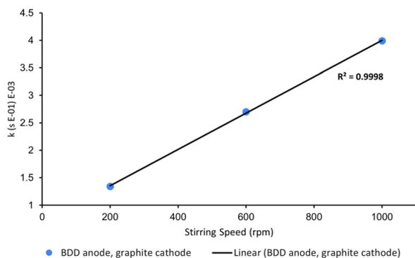
Fig. 8 Effect of varying stirring speed on the first-order rate constants for the decolorisation of AO7 at 10 min. Conditions: [AO7] = 100  $\mu$ M, boron-doped diamond anode, graphite cathode, [Na<sub>2</sub>S<sub>2</sub>O<sub>8</sub>] = 14 mM,  $I$  = 5 mA.
