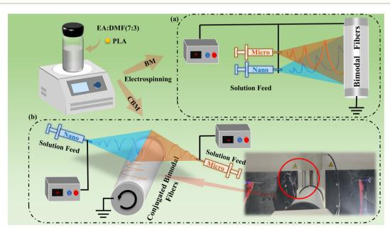
Fig. 1 Schematic illustration of the bimodal PLA membranes. (a) The double-spinneret parallel electrospinning process, and (b) the conjugated bimodal electrospinning membrane that with 3d structures.
