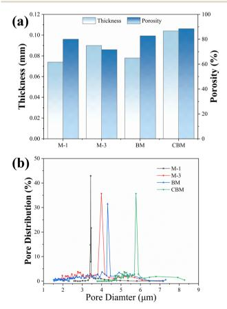
Fig. 3 (a) Porosity and thickness, and (b) the distribution of pore size of M-1, M-2, BM, and CBM.
