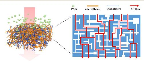
Fig. 7 A schematic explaining the filtration process of CBM for PMs.
