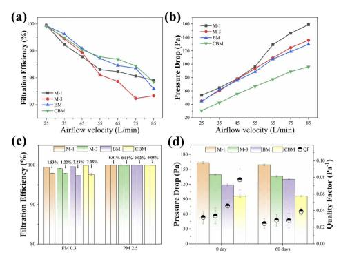
Fig. 5 (a) Filtration efficiency under various air flow rates, (b) pressure drop under various air flow rates of M-1, M-2, BM, and CBM. (c) Filtration efficiency after storage on 60 days with PM 0.3 and PM 2.5, (d) pressure drop and quality factor after storage on 60 days with PM 0.3.
