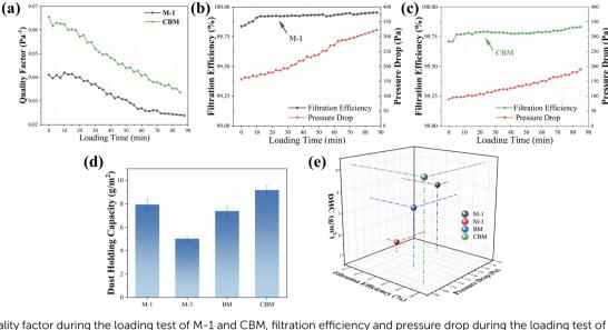
Fig. 6 (a) Quality factor during the loading test of M-1 and CBM, filtration efficiency and pressure drop during the loading test of (b) M-1 and (c) CBM. (d) Dust holding capacity against NaCl aerosol particles, (e) comparison of comprehensive filtration performance of M-1, M-3, BM and CBM.
