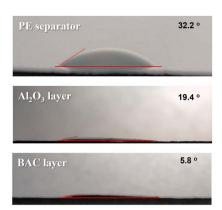
Fig. 3 Contact angle measurement of the bare PE separator (a), PE separator coated with  $Al_2O_3$  layer (b), and PE separator coated with BAC layer using 1 M LiTFSI in DOL/DME.
