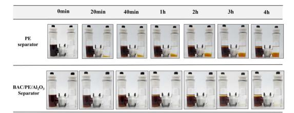
Fig. 7 Digital images of LiPS dissolution test in H-type cells with the PE and BAC/PE/Al<sub>2</sub>O<sub>3</sub> separator for 4 hours.
