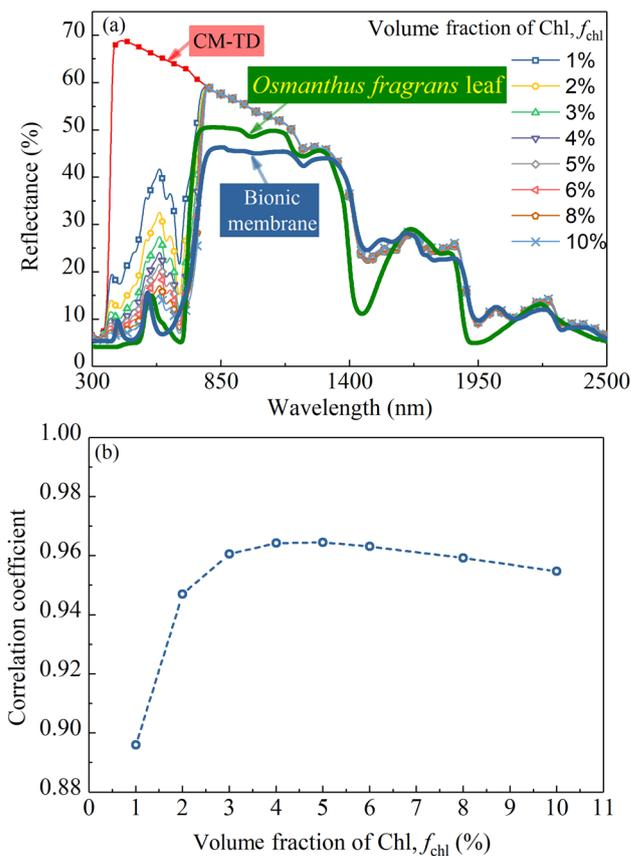
Fig. 10 (a) Calculated reflectances of CM-Chl/TD with  $f_{chl}$  ranging from 1%–10% (thickness is 0.3 mm, and  $f_{td}$  is 0.7%), (b) correlation coefficients between the reflectances of the above CM-Chl/TD samples and the *Osmanthus fragrans* leaf.
