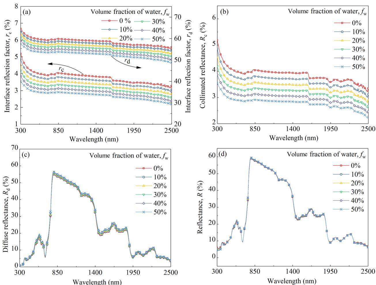
Fig. 12 (a) Calculated interface reflection coefficients, (b) collimated reflectances, (c) diffuse reflectances and (d) total reflectances of the CM-Chl/TD samples with  $k_w$  equal to zero and different refractive indexes (thickness is 0.3 mm,  $f_{td}$  and  $f_{chl}$  are 0.7% and 5%, respectively).
