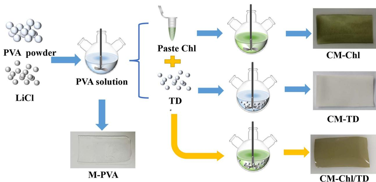
Fig. 1 Schematic diagram of the specific preparation process of the camouflage membrane.
