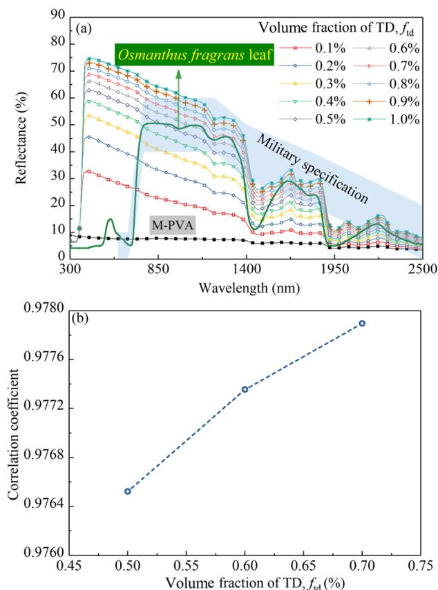
Fig. 8 (a) Calculated reflectances of CM-TD (thickness is 0.3 mm) with different  $f_{td}$  ranging from 0.1% to 1%, (b) correlation coefficients between the spectral reflectances of the CM-TD with  $f_{td}$  ranging from 0.5% to 0.7% and the *Osmanthus fragrans* leaf.
