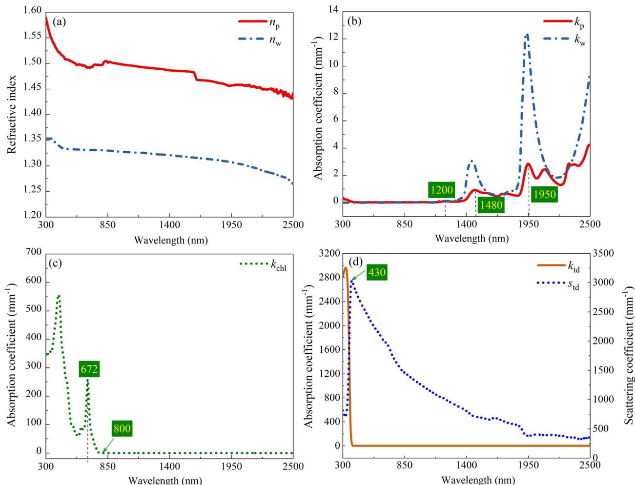
Fig. 6 (a) Refractive indexes and (b) absorption coefficients of M-PVA and water,<sup>27</sup> (c) absorption coefficient of Chl, (d) absorption and scattering coefficients of TD particle.
