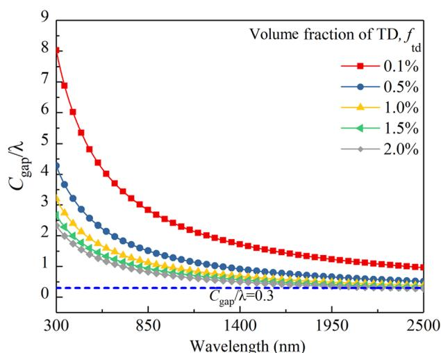
Fig. 4  $C_{\text{gap}}/\lambda$  of the membranes containing different  $f_{\text{td}}$ .
