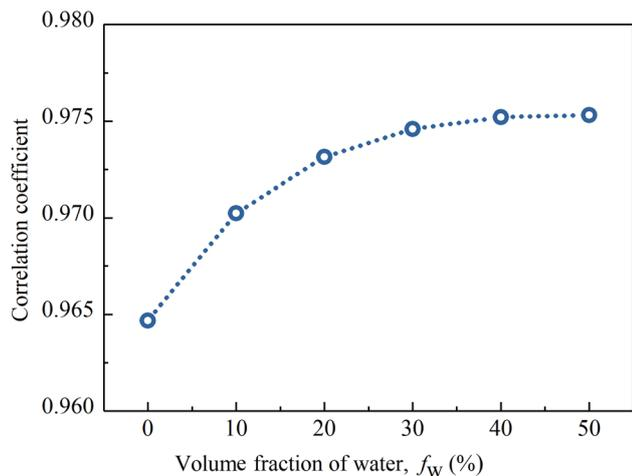
Fig. 13 Correlation coefficients between the reflectances of the CM-Chl/TD samples (thickness is 0.3 mm,  $f_{td}$  and  $f_{chl}$  are 0.7% and 5%, respectively) containing different  $f_w$  and the *Omanthus fragrans* leaf.
