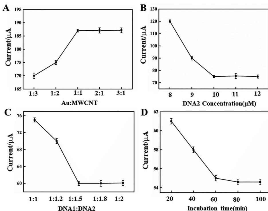
Fig. 4 The effect of (A) molar ration of Au NPs : MWCNTs, (B) amount of DNA2, (C) amount of DNA1, and (D) incubation time of DNA2 and DNA1-MB in CV. Data are presented as mean  $\pm$  SD ( $n = 5$  independent experiments).
