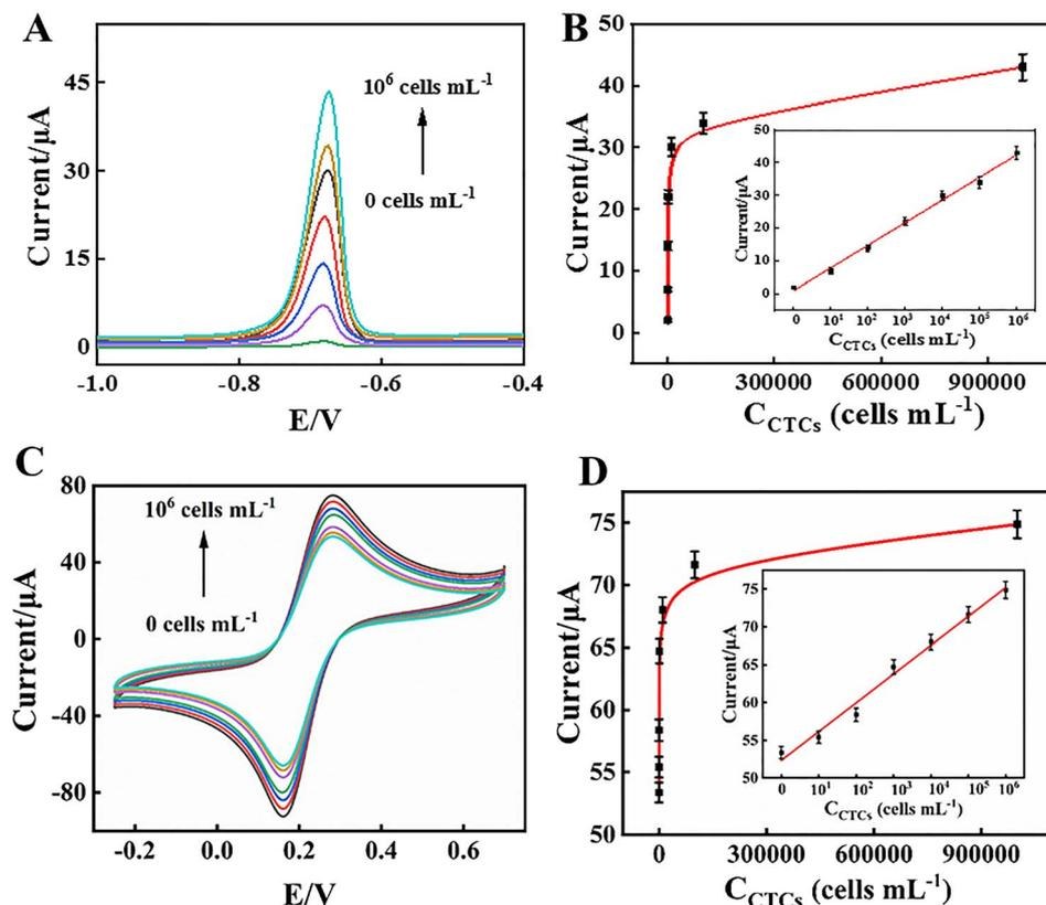
Fig. 5 (A) ASV and (C) CV responses of the electrochemical biosensor incubated with different concentrations of MCF-7 cells in 0.01 M phosphate buffer (pH = 6.5; 0, 10, 1 × 10<sup>2</sup>, 1 × 10<sup>3</sup>, 1 × 10<sup>4</sup>, 1 × 10<sup>5</sup>, 1 × 10<sup>6</sup> cells per mL); (B) and (D) calibration curve of the cytosensor for MCF-7 cells.
