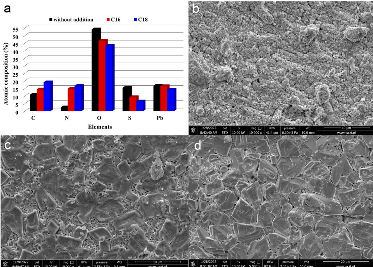
**Fig. 3** Chemical composition (a) and SEM images (b–d) of positive current collectors, derived from batteries containing unmodified (b) and ILs-modified ((c) C16, (d) C18) sulfuric acid electrolytes. Results represents the state after electrodes soaking, formation process and stages 1–3 of battery testing (Table 2).
