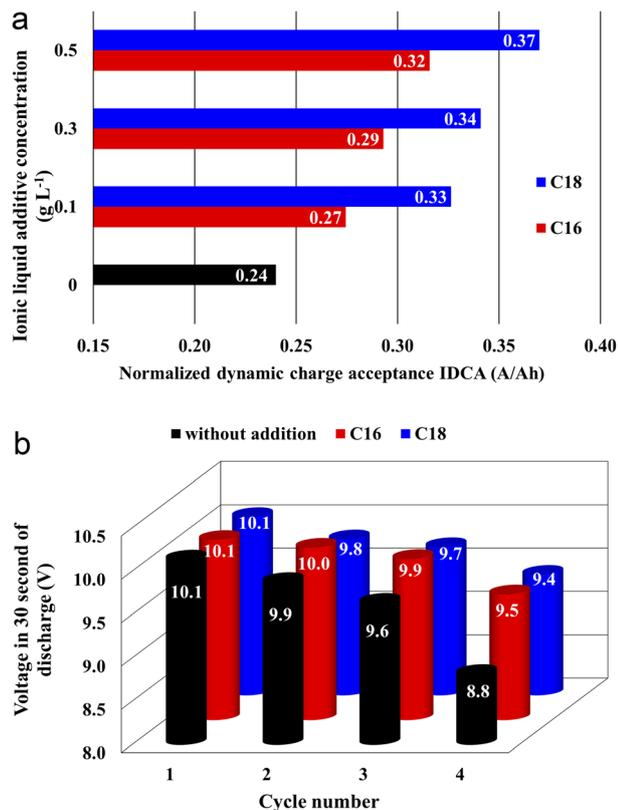
Fig. 5 The normalized dynamic charge acceptance (DCA) capacity (a) and voltage value in 30 second of discharge during corrosion resistance test (b). The results concern lead–acid batteries containing unmodified (black) and ILs-modified (red and blue) sulfuric acid electrolytes.
