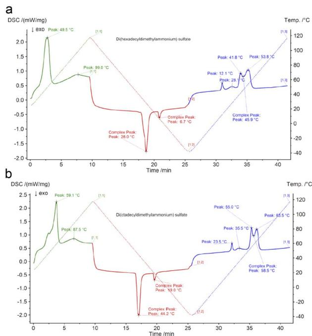
Fig. 1 Thermal transition temperatures for (a) di(hexadecyldimethylammonium) sulphate and (b) di(octadecyldimethylammonium) sulphate.
