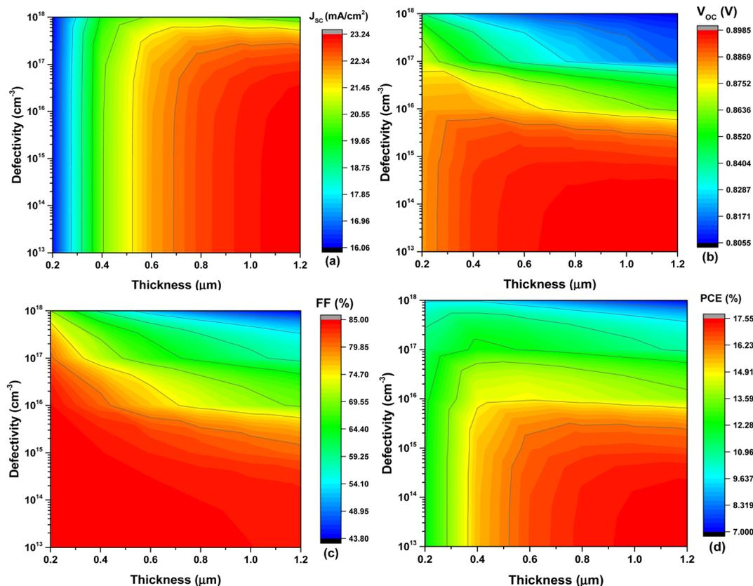
Fig. 4 The contour plotting of the perovskite material *i.e.*, MAPbI<sub>3</sub> for high output parameters at the optimized temperature and doping conditions.
