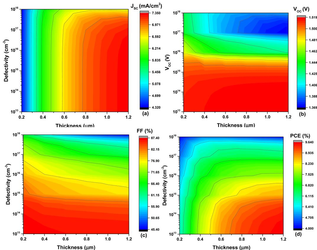
Fig. 6 The contour plotting of the perovskite material *i.e.*, MAPbBr<sub>3</sub>, for high output parameters at the optimized temperature and doping conditions.
