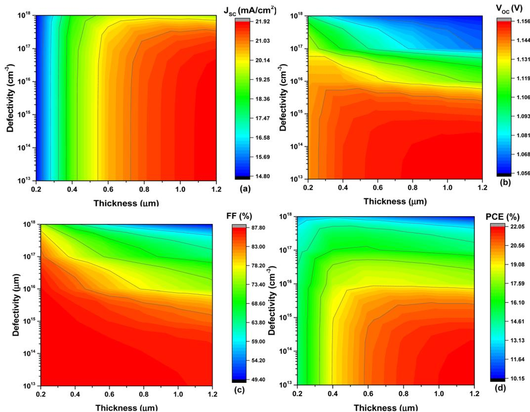
Fig. 5 The contour plotting of the perovskite material, *i.e.*, MAPbI<sub>2</sub>Br, for high output parameters at the optimized temperature and doping conditions.
