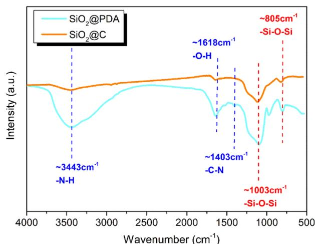
Fig. 4 FTIR of the precursor SiO<sub>2</sub>@PDA and the conductive carbon nanospheres.
