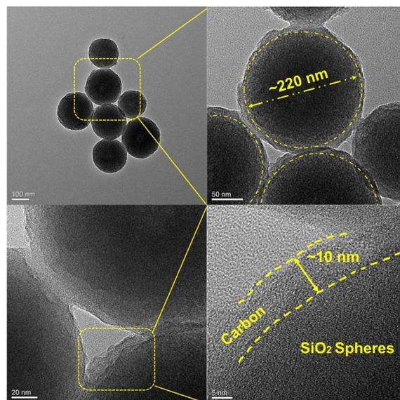
Fig. 7 TEM images of conductive carbon nanospheres.
