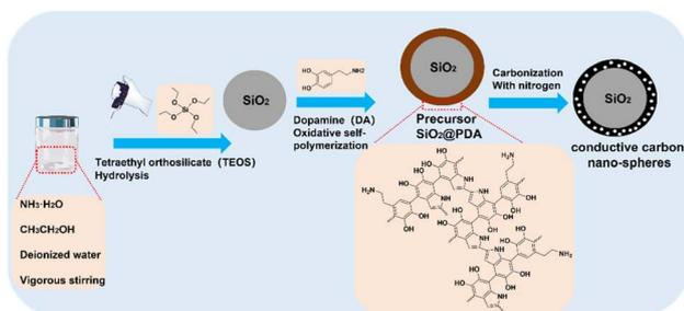
Fig. 1 Schematic diagram of the synthesis approach.
