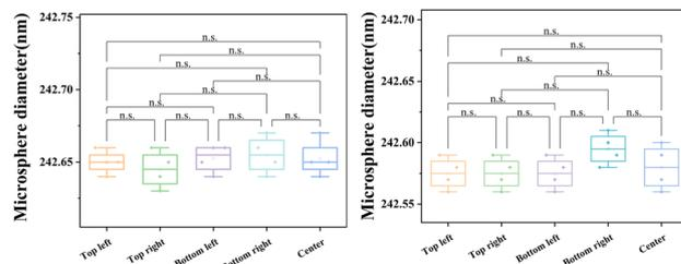
**Fig. 11** One-way ANOVA plot of photographing positions for measured diameters in the X-axis direction and the Y-axis direction. n.s. means  $p$ -value  $> 0.05$  (each scatter in the bar represents a sample).
