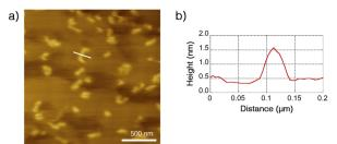
Fig. 4 (a) Dynamic-mode AFM image (2.0  $\times$  2.0  $\mu m^2$  on a HOPG substrate) of Ru-PP and (b) height profile on a cross-section of the white line.
