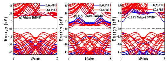
Electronic band structures of (a) pristine SWBNNT (b) B-doped SWBNNT and (c) N-doped SWBNNT.
