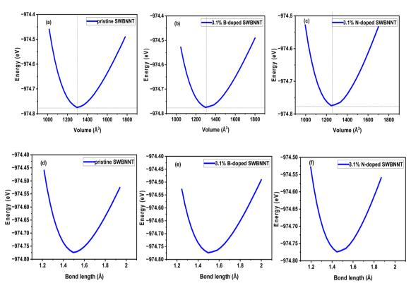
Fig. 2 Variation of energy with volumes of (a) pristine SWBNNT (b) B-doped (3.1%) SWBNNT and (c) N-doped (3.1%) SWBNNT. Energy variation with bond lengths of (d) pristine SWBNNT (e) B-doped (3.1%) SWBNNT and (f) N-doped (3.1%) SWBNNT.
