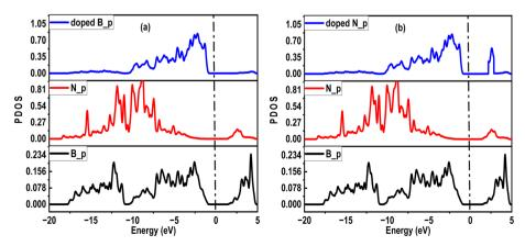
Fig. 6 PDOS diagrams of (a) B-doped SWBNNT (b) N-doped SWBNNT.
