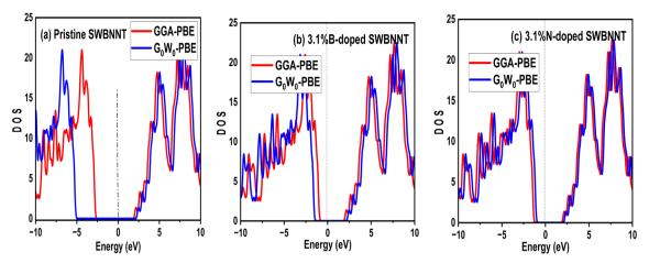
Fig. 5 Electronic density of states of (a) pristine SWBNNT (b) B-doped SWBNNT and (c) N-doped SWBNNT.
