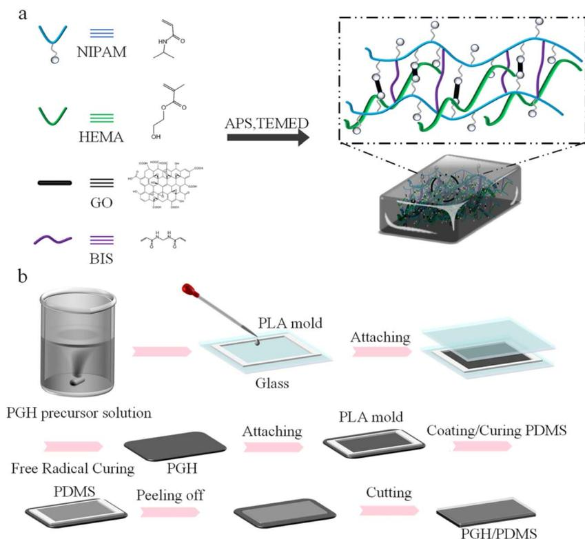
Fig. 1 (a) Schematic illustration for the preparation of PNIPAM-based composite hydrogel. (b) Schematic illustration of the preparation process of the PGH/PDMS photothermal bilayer actuator.
