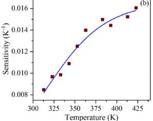
Fig. 8 UC-based ratiometric temperature sensing using  $\alpha$ -NaYF<sub>4</sub>:-Yb<sup>3+</sup>/Er<sup>3+</sup> nanophosphor: (a) plot of ln(FIR) (using 523 and 548 nm emission) as a function of the inverse absolute temperature, (b) temperature sensitivity as a function of temperature.
