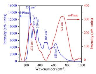
Fig. 3 Raman spectra of  $\alpha$ -NaYF $_4$ :Yb $^{3+}$ /Er $^{3+}$  and  $\beta$ -NaYF $_4$ :Yb $^{3+}$ /Er $^{3+}$  nanophosphors.
