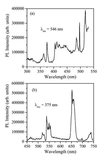
Fig. 4 (a) PL excitation spectrum of  $\beta$ -NaYF<sub>4</sub>:Yb<sup>3+</sup>/Er<sup>3+</sup> monitored at 546 nm emission wavelength. (b) The PL emission spectrum of  $\beta$ -NaYF<sub>4</sub>:Yb<sup>3+</sup>/Er<sup>3+</sup> was monitored at 375 nm excitation wavelength.
