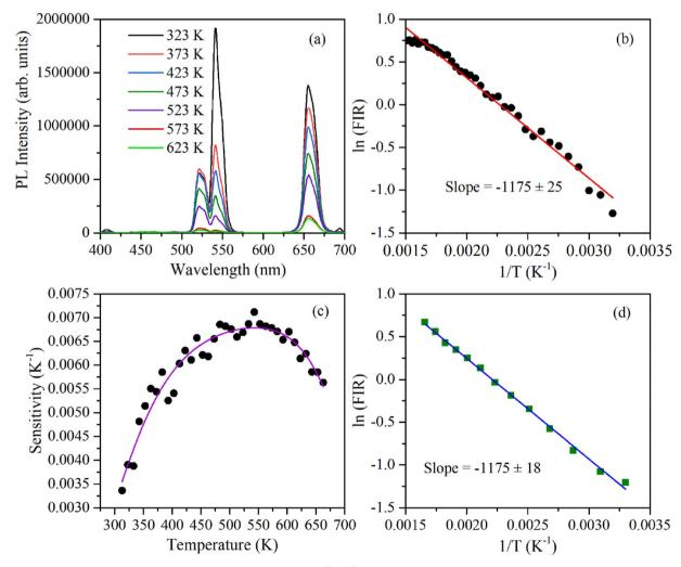
Fig. 7 UC-based ratiometric temperature sensing using  $\beta$ -NaYF<sub>a</sub>:Yb<sup>3+</sup>/Er<sup>3+</sup> phosphor: (a) UC emission spectra measured between 300 and 650 K, (b) plot of ln(FIR) (using 523 and 548 nm emission) as a function of the inverse absolute temperature during heating, (c) temperature sensitivity as a function of temperature, (d) plot of ln(FIR) as a function of the inverse absolute temperature during cooling.
