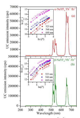
Fig. 6 UC emission spectra of (a) α-NaYF<sub>4</sub>:Yb<sup>3+</sup>/Er<sup>3+</sup> and (b) β-NaYF<sub>4</sub>:Yb<sup>3+</sup>/Er<sup>3+</sup> were recorded using continuous-wave diode laser radiating at 976 nm wavelength. Inset to the Figures shows ln(l) and ln(P) plot at different emission wavelengths.
