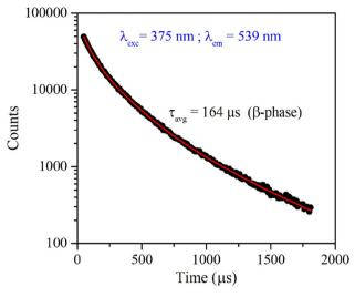
Fig. 5 Time-resolved PL of  $\beta$ -NaYF<sub>4</sub>:Yb<sup>3+</sup>/Er<sup>3+</sup> phosphor monitored at 375 nm excitation and 539 nm emission wavelength, respectively.
