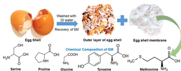
Fig. 1 Separation of calcite-rich outer eggshell and inner membrane from the raw eggshell and the chemical composition of EM.
