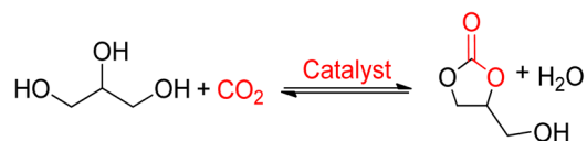
Scheme 7 Glycerol carbonate (GC) obtained from glycerol and CO 2 (reproduced from ref. 82 with permission from RSC copyright 2021).
