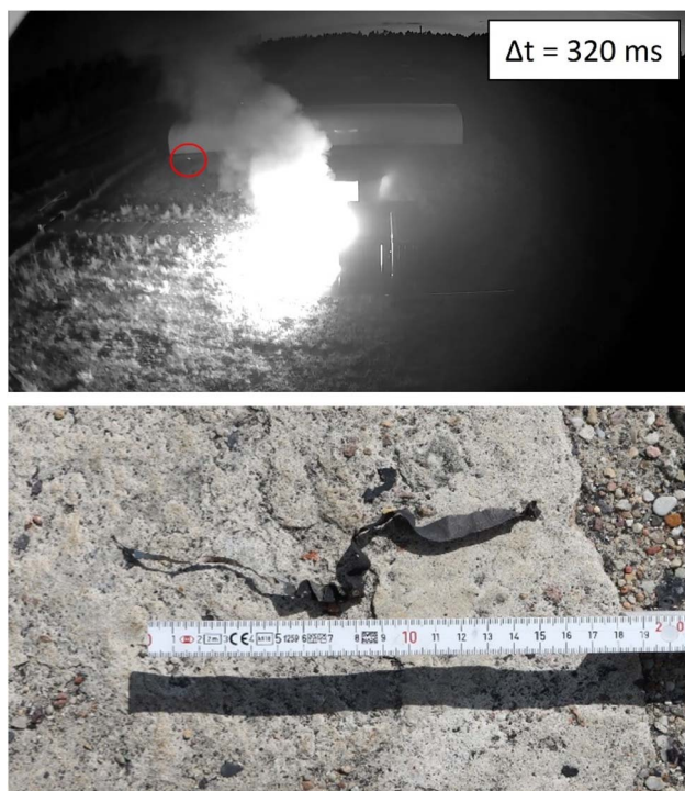
Fig. 14 Test #11, top: picture taken from a video recorded in night vision mode, \Delta t = 320 ms after TR, flyaway fragment red circled, bottom: fragment, length l = 17 cm found at a distance of l \approx 33.2 m.
