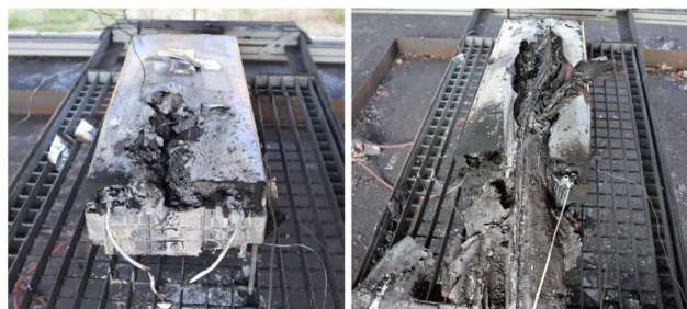
Fig. 11 Damaged test modules from overheating test #10 (left) and overcharging test #11 (right).
