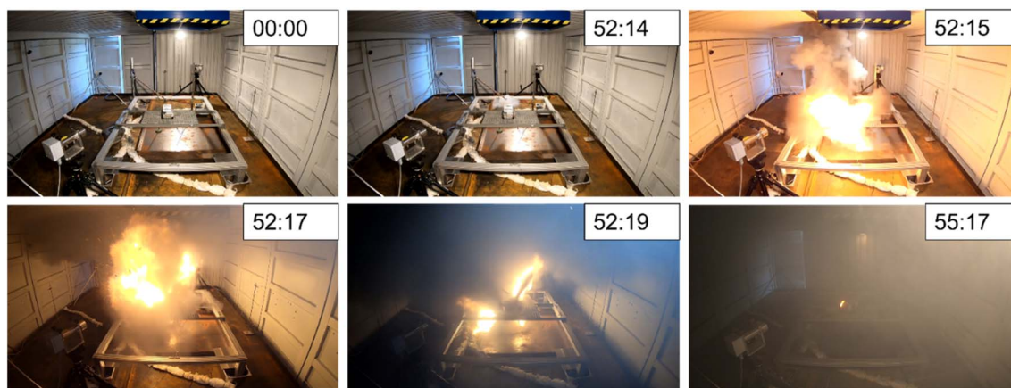
Fig. 7 Time sequence of 2.65 kWh module in test #07 during TR with released gas and igniting jet flame.
