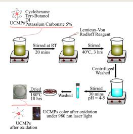
Fig. 2 Process of NaYF<sub>4</sub>:Tm, Yb surface modification.
