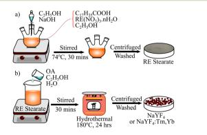
Fig. 1 Schema of preparation (a) stearate salts of REs and (b)  $NaYF_4$ :Tm, Yb UCMPs.
