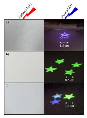
Fig. 12 Screen printing patterns of NaYF<sub>4</sub>:1Tm,30Yb (a); NaYF<sub>4</sub>:1-Er,20Yb (b); the combination of NaYF<sub>4</sub>:1Tm,30Yb and NaYF<sub>4</sub>:1Er,20Yb with a ratio of 90:10 (% w/w) (c).
