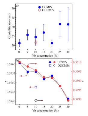
Fig. 4 (a) Crystallite size and (b) lattice constants a, c of NaYF<sub>4</sub> as a function of Yb concentrations.
