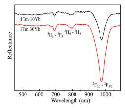
Fig. 8 DRS spectra of 1Tm10Yb and 1Tm30Yb powders.
