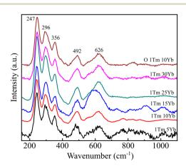
Fig. 5 Raman spectra of NaYF<sub>4</sub>:1TmxYb with x = 5, 10, 15, 20, 25, and 30 mol% & OUCMPs 1Tm10Yb.
