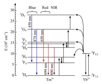
Fig. 11 The UC emission mechanism of NaYF<sub>4</sub>:Tm, Yb
