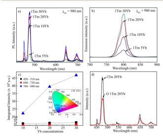
Fig. 9 PL spectra of NaYF<sub>4</sub>:1Tm, xYb with x = 5, 10, 20 and 30 mol% (a and b); integrated intensity and CIE of samples (c); PL spectra of 1Tm20Yb and O1Tm20Yb (d)
