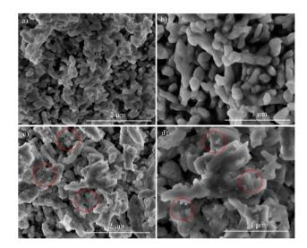
SEM images of 1Tm20Yb (a and b) and 1Tm30Yb (c and d)
