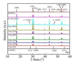
Fig. 3 XRD patterns of NaYF<sub>4</sub>:1TmxYb with x = 5, 10, 15, 20, 25, and 30 mol% & OUCMPs 1Tm10Yb.
