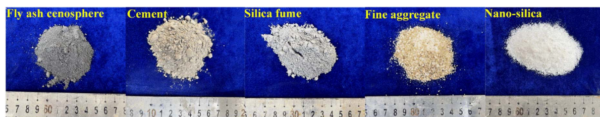
Fig. 1 Appearances of the five basic materials employed in this study.
