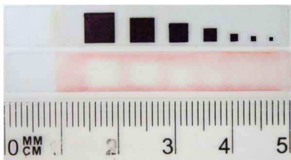
Fig. 7 Photopattern containing patterns of different size photolithographically immobilized on a substrate and photomask used for the photopatterning.
