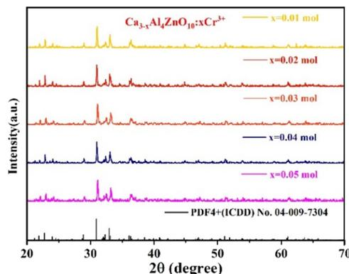
Fig. 1 XRD patterns of the synthesized CAZ samples.
