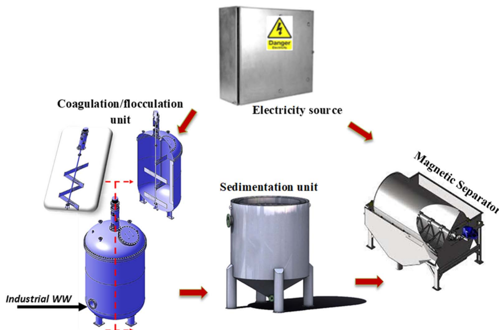
Fig. 11 Main proposed large-scale treatment units employed by MN-CFs for industrial effluent decontamination.
