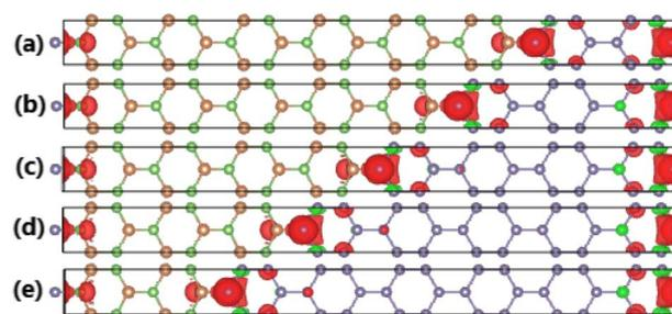
Fig. 15 Spin density (red surface: spin-up state; green surface: spin-down state; iso-surface value:  $0.0005 e \text{ \AA}^{-3}$ ) in  $(\text{Ge})_m-(\text{AsSb})_{8-m}$  lateral heterostructures with (a)  $m = 2$ , (b)  $m = 3$ , (c)  $m = 4$ , (d)  $m = 5$ , and (e)  $m = 6$ .
