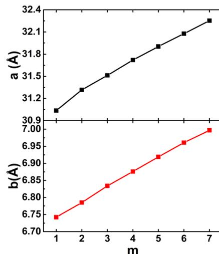
Fig. 6 Lattice constants of armchair-interline  $(\text{Ge})_m\text{-(AsSb)}_{8-m}$  lateral heterostructures.
