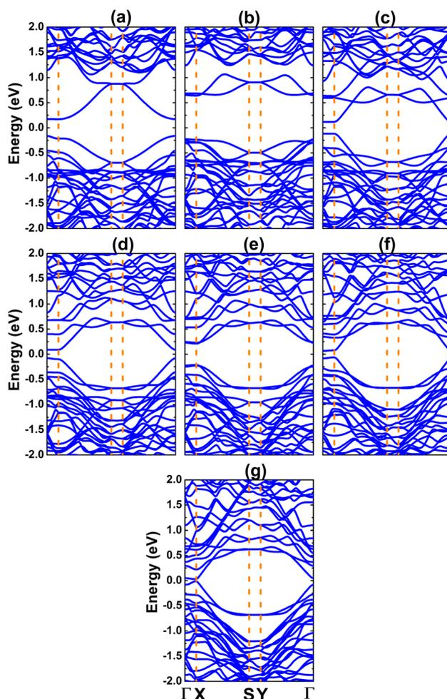
Fig. 7 Electronic band structure (blue curves: non-spin-polarization) of armchair-interline  $(\text{Ge})_m\text{-(AsSb)}_{8-m}$  lateral heterostructures with (a)  $m = 1$ , (b)  $m = 2$ , (c)  $m = 3$ , (d)  $m = 4$ , (e)  $m = 5$ , (f)  $m = 6$ , and (g)  $m = 7$ .
