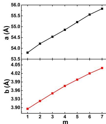
Fig. 11 Lattice constants of zigzag-interline  $(\text{Ge})_m-(\text{AsSb})_{8-m}$  lateral heterostructures.
