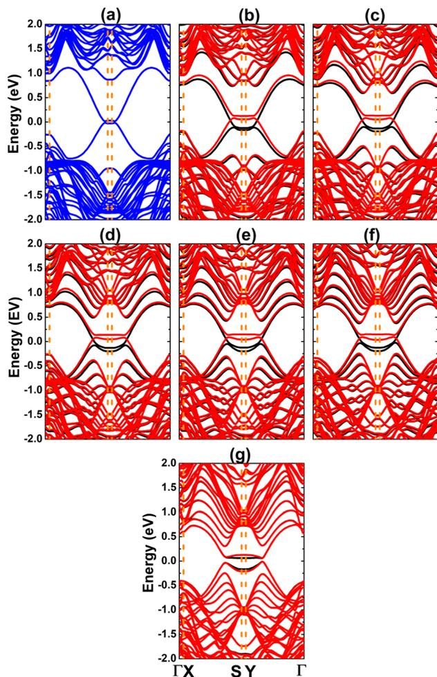
Fig. 12 Electronic band structure (blue curve: non-spin-polarization; black curve: spin-up; red curve: spin-down) of zigzag-interline  $(\text{Ge})_m-(\text{AsSb})_{8-m}$  lateral heterostructures with (a)  $m = 1$ , (b)  $m = 2$ , (c)  $m = 3$ , (d)  $m = 4$ , (e)  $m = 5$ , (f)  $m = 6$ , and (g)  $m = 7$ .
