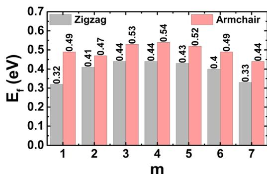
Fig. 5 Formation energy of  $(\text{Ge})_m\text{-(AsSb)}_{8-m}$  lateral heterostructures with armchair- and zigzag-interline.
