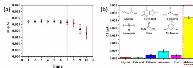
**Fig. 7** The responses of the CuO/MIP electrode in tests of its reusability for melamine detection (a) and its selectivity to different compounds such as glycine, uric acid, thiourea, ammonia, urea, and melamine (b).
