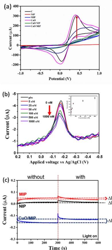
Fig. 5 Response analysis of surface-modified electrodes: cyclic voltammogram of the different modified electrodes using 0.05 M ( $[K_4Fe(CN)_6]$ ) in 0.1 M PBS (a), differential pulse voltametric response in different concentrations of melamine at 0–100.0 nM (b), relationship between the DPV current and melamine concentration (inset) and amperometry current response of 100.0 nM melamine with different modified electrodes (c) using a constant light intensity of  $3 \text{ mW cm}^{-2}$ .
