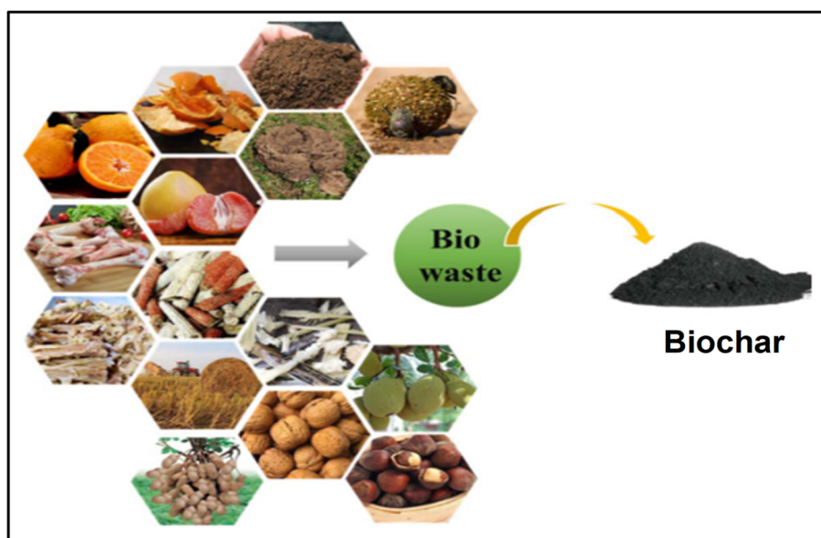
Fig. 11 Schematic diagram showing the conversion of agro-waste into biochar for heavy metals removal from aqueous systems carbon (this figure has been adapted from Wang et al. 31 with permission from RSC, copyright 2023).
