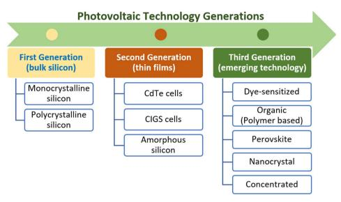
Fig. 1 Three generations of PV cells.
