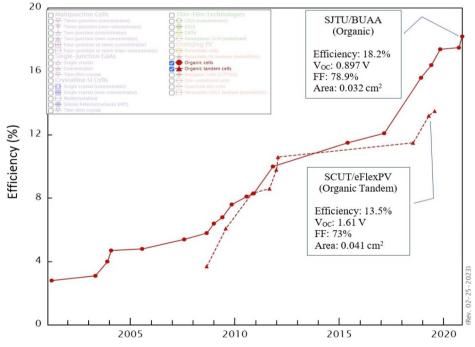
Fig. 8 Conversion efficiencies for OPV cells from 2001 to 2021. 157
