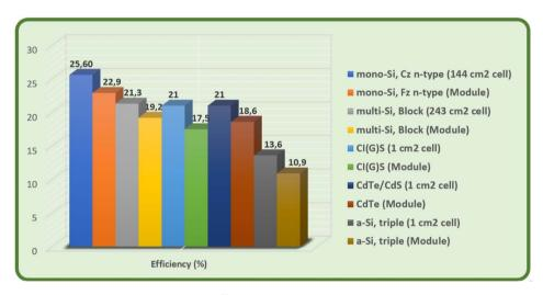
Fig. 2 Efficiency of silicon-based technology in laboratories.<sup>37</sup>
