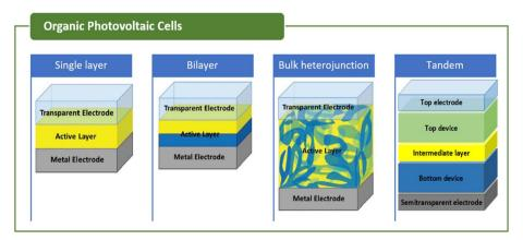
Fig. 5 Device structure of OPV cells
