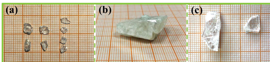
Fig. 3 (a) Y_2Mo_4O_{15} grains obtained by spontaneous crystallization; (b) seedless growth of Y_2Mo_4O_{15} single crystal; (c) photo of Y_2Mo_4O_{15} single crystal after optimizing seed crystal, flux system, and viscosity.
