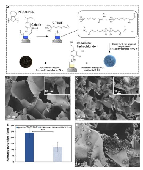
Fig. 1 Morphological evaluation of the synthesized scaffolds. (A) Schematic of fabrication process. (B) FE-SEM micrographs of gelatin-PEDOT:PSS and (C and D) PDA-coated gelatin-PEDOT:PSS constructs. (E) Average pore size of modified and un-modified scaffolds. (Difference is extremely statistically significant (\*\*\*p < 0.001)).
