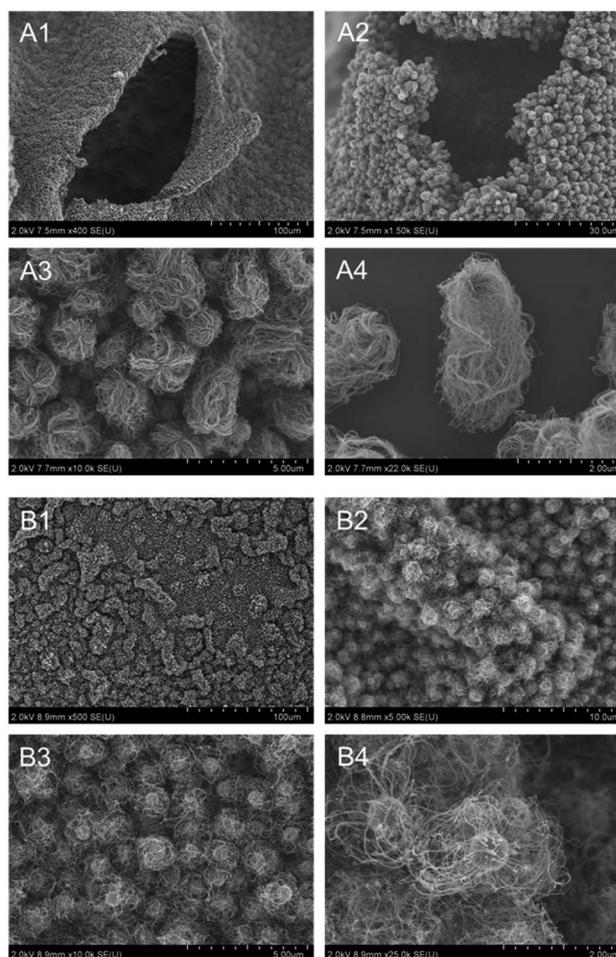
Fig. 12 SEM images of CNT-hairs at different magnifications obtained using (A) s20-FeO<sub>x</sub>/ZrO<sub>2</sub>-M and (B) i20-FeO<sub>x</sub>/ZrO<sub>2</sub>-M catalysts at 730 °C under pressure of 65 Pa with a 10 sccm ethyne gas flow for 10 s.
