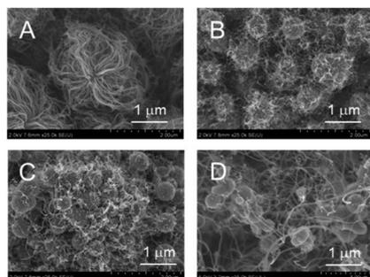
Fig. 5 SEM images of CNT-hair obtained using different catalysts, including (A) s20-FeO<sub>x</sub>/ZrO<sub>2</sub>-M, (B) s20-CoO<sub>x</sub>/ZrO<sub>2</sub>-M, (C) s20-NiO<sub>x</sub>/ZrO<sub>2</sub>-M and (D) s50-FeO<sub>x</sub>/CeO<sub>2</sub>-M at 730 °C under pressure of 65 Pa with a 10 sccm ethyne gas flow for 10 s.
