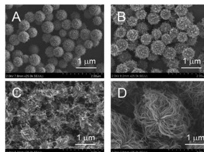
Fig. 8 SEM images of products obtained using s20-FeO<sub>x</sub>/ZrO<sub>2</sub>-M catalysts with different reaction times at 730 °C under pressure of 65 Pa with a 10 sccm ethyne gas flow. (A) 0.5 s, (B) 1 s, (C) 3 s and (D) 10 s (the same as Fig. 5A).
