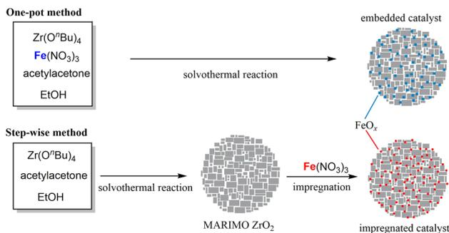
Fig. 2 One-pot solvothermal synthesis of FeO<sub>x</sub> catalyst embedded in ZrO<sub>2</sub> MARIMO (top) and step-wise preparation of FeO<sub>x</sub> catalyst impregnated in MARIMO ZrO<sub>2</sub> (bottom).
