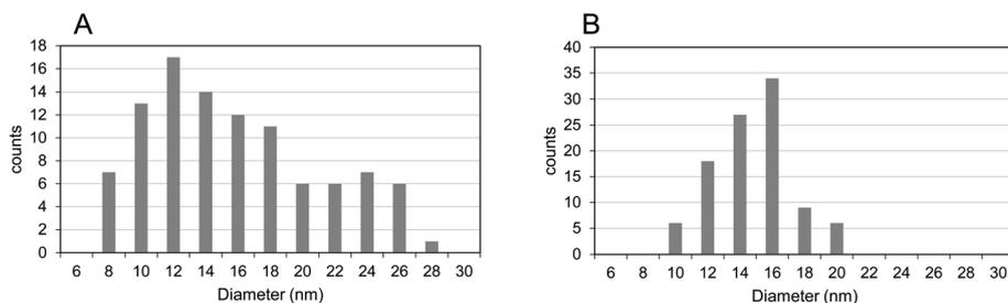
Fig. 15 Diameter distributions of CNT-hairs obtained using (A) s20-FeO<sub>x</sub>/ZrO<sub>2</sub>-M catalyst and (B) i20-FeO<sub>x</sub>/ZrO<sub>2</sub>-M catalyst at 730 °C under pressure of 65 Pa with a 10 sccm ethyne gas flow for 10 s.
