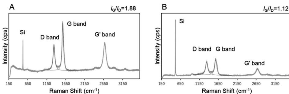
Fig. 16 Raman spectra of CNT-hairs obtained using (A) s20-FeO<sub>x</sub>/ZrO<sub>2</sub>-M and (B) i20-FeO<sub>x</sub>/ZrO<sub>2</sub>-M catalysts at 730 °C under pressure of 65 Pa with a 10 sccm ethyne gas flow for 10 s. The Si peaks at 520 cm<sup>-1</sup> were observed in both samples on the th-SiO<sub>2</sub> substrates on which MARIMO catalysts were drop-cast.
