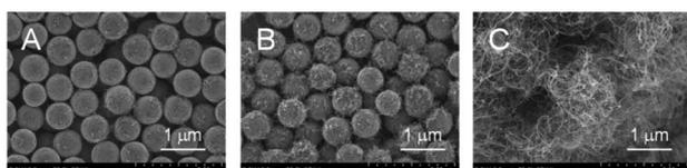
Fig. 10 SEM images of products obtained using catalysts with different quantities of FeO<sub>x</sub>. (A) i5-FeO<sub>x</sub>/ZrO<sub>2</sub>-M, (B) i10-FeO<sub>x</sub>/ZrO<sub>2</sub>-M and (C) i20-FeO<sub>x</sub>/ZrO<sub>2</sub>-M (the same as Fig. 9B) at 730 °C under pressure of 65 Pa with a 10 sccm ethyne gas flow for 10 s.
