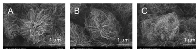
Fig. 7 SEM images of CNT-hair obtained using s20-FeO<sub>x</sub>/ZrO<sub>2</sub>-M catalysts at temperatures of (A) 670 °C, (B) 730 °C (the same as Fig. 5A) and (C) 760 °C under pressure of 65 Pa with a 10 sccm ethyne gas flow for 10 s.
