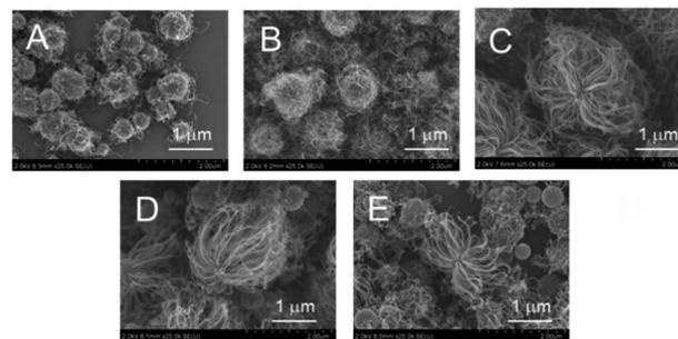
Fig. 6 SEM images of CNT-hair obtained using different quantities of catalysts, including (A) s5-FeO<sub>x</sub>/ZrO<sub>2</sub>-M, (B) s10-FeO<sub>x</sub>/ZrO<sub>2</sub>-M, (C) s20-FeO<sub>x</sub>/ZrO<sub>2</sub>-M (the same as Fig. 5A), (D) s30-FeO<sub>x</sub>/ZrO<sub>2</sub>-M and (E) s50-FeO<sub>x</sub>/ZrO<sub>2</sub>-M at 730 °C under pressure of 65 Pa with a 10 sccm ethyne gas flow for 10 s.
