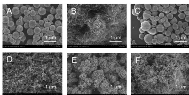
Fig. 9 SEM images of products obtained using FeO<sub>x</sub> catalysts supported on different metal oxides. (A) i20-FeO<sub>x</sub>/TiO<sub>2</sub>-M, (B) i20-FeO<sub>x</sub>/ZrO<sub>2</sub>-M, (C) i20-FeO<sub>x</sub>/SnO<sub>2</sub>-M, (D) i20-FeO<sub>x</sub>/CeO<sub>2</sub>-M, (E) i20-FeO<sub>x</sub>/ZrO<sub>2</sub>-W and (F) i20-FeO<sub>x</sub>/ZrO<sub>2</sub>-U at 730 °C under pressure of 65 Pa with a 10 sccm ethyne gas flow for 10 s.
