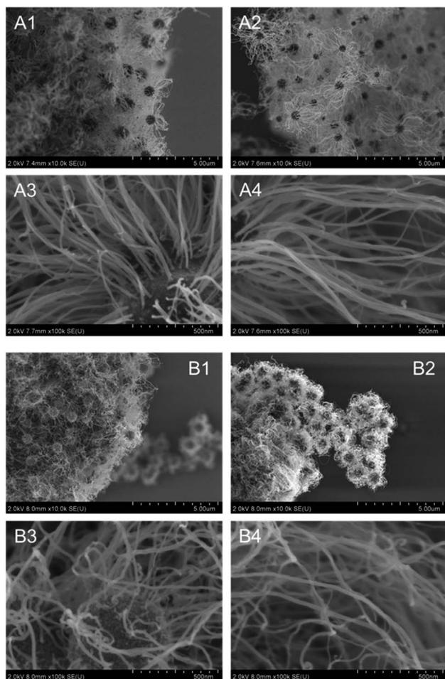
Fig. 13 SEM images of CNT-hairs at different magnifications obtained using (A)  $s20\text{-FeO}_x/\text{ZrO}_2\text{-M}$  and (B)  $i20\text{-FeO}_x/\text{ZrO}_2\text{-M}$  catalysts at  $730^\circ\text{C}$  under pressure of 65 Pa with a 10 sccm ethyne gas flow for 10 s.
