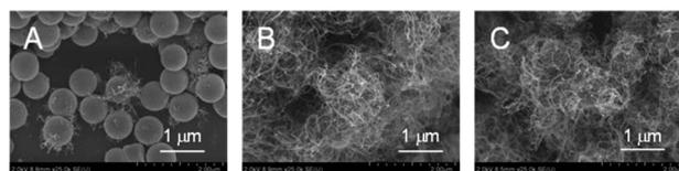
Fig. 11 SEM images of products obtained using i20-FeO<sub>x</sub>/ZrO<sub>2</sub>-M at different temperatures. (A) 670 °C, (B) 730 °C (the same as Fig. 9B) and (C) 760 °C under pressure of 65 Pa with a 10 sccm ethyne gas flow for 10 s.
