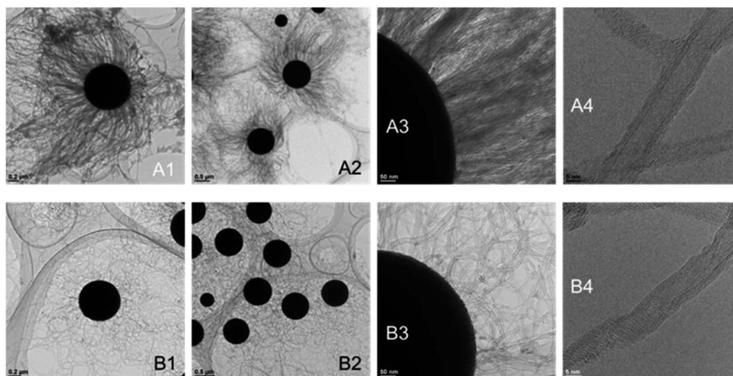
Fig. 14 TEM images of CNT-hairs at different magnifications obtained using (A)  $s20\text{-FeO}_x/\text{ZrO}_2\text{-M}$  and (B)  $i20\text{-FeO}_x/\text{ZrO}_2\text{-M}$  catalysts at  $730^\circ\text{C}$  under pressure of 65 Pa with a 10 sccm ethyne gas flow for 10 s.
