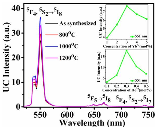
Fig. 4 Upconversion emission spectra for as-synthesized & annealed samples in 520–760 nm range. The inset (up) shows the intensity variation for different Yb<sup>3+</sup> ion concentrations and inset (down) shows intensity variation for different Ho<sup>3+</sup> ion concentrations.
