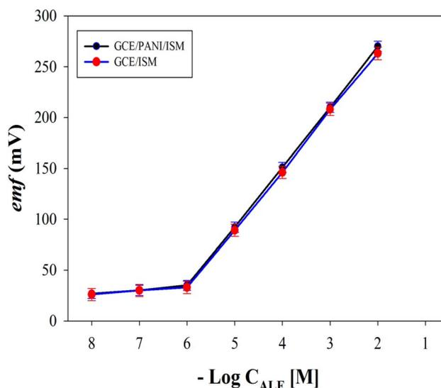
Fig. 3 Profile of the potential in mV versus -log molar concentration of ALF in M obtained with sensors 1 and 2.
