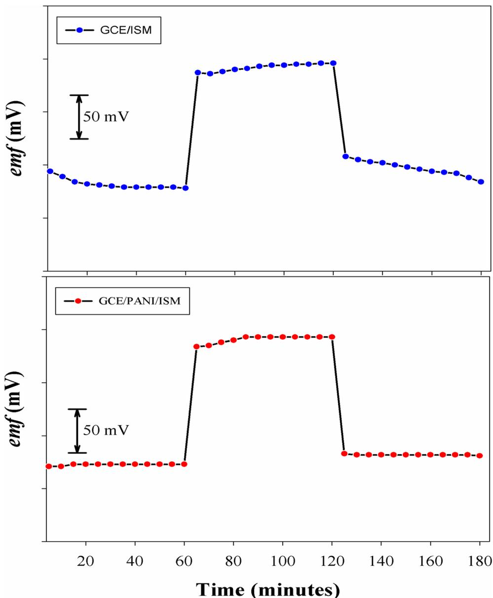
Fig. 4 Water layer test for both GCE/PANI/ISM (sensor 1) and GCE/ISM (sensor 2). The electromotive force (*emf*) was recorded successively in  $1.0 \times 10^{-3} \text{ mol L}^{-1}$  ALF,  $1.0 \times 10^{-2} \text{ mol L}^{-1}$  antazoline HCl, and then  $1.0 \times 10^{-3} \text{ mol L}^{-1}$  ALF using PANI and control SC-ISEs.
