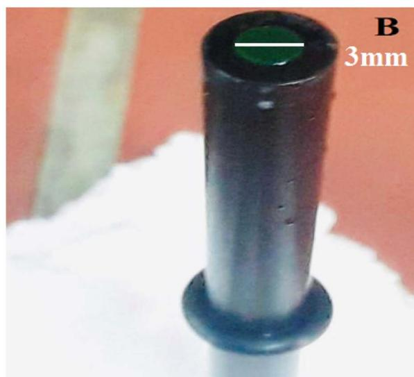
Fig. 2 (A) Electrochemical polymerization of PANI at GCE surface versus Ag/AgCl reference electrode using 0.1 M aniline monomer in 0.1 M H<sub>2</sub>SO<sub>4</sub> solution by applying potential cycle  $-0.1$  to  $1.0$  V vs. Ag/AgCl at scan rate  $50$  mV s<sup>-1</sup> for 10 cycles. (B) Photographic image of GCE/PANI modified electrode.
