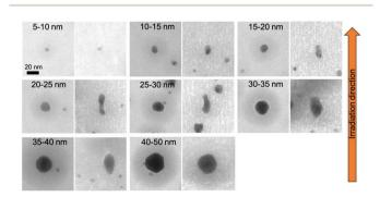
Fig. 8 TEM images of elongated Au nanoparticles sandwiched between two 50 nm ALD-Al $_2$ O $_3$  layers and irradiated with 50 MeV  $^{127}$ I at 5  $\times$  10 $^{13}$  ions per cm $^2$  before (left) and after (right) the irradiation.
