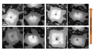
Fig. 7 TEM images of fabricated nanorods with different orientations embedded in 100 nm ALD-SiO $_2$  and irradiated with 50 MeV  $^{127}$ I at 2  $\times$  10 $^{14}$  ions per cm $^2$  before (left) and after (right) the irradiation. (a) Length = 33.2 nm and diameter = 22.6 nm, (b) length = 37.1 nm and diameter = 25.1 nm, (c) length = 35.0 nm and diameter = 24.4 nm, and (d) length = 62.8 nm and diameter = 29.2 nm before (left) and after (right) irradiation.
