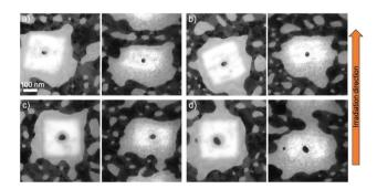
Fig. 4 TEM images of fabricated nanorods with different orientations embedded in 100 nm ALD-SiO $_2$  and irradiated with 50 MeV  $^{127}$ I at 5  $\times$   $10^{13}$  ions per cm $^2$  before (left) and after (right) the irradiation. (a) Length = 35.9 nm and diameter = 24.0 nm, (b) length = 42.1 nm and diameter = 29.9 nm, (c) length = 51.9 nm and diameter = 37.1 nm, and (d) length = 58.2 nm and diameter = 36.0 nm. These nanorods did not manage to re-orient along the ion beam direction.
