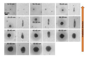
Fig. 9 TEM images of elongated Au nanoparticles sandwiched between two 50 nm ALD-Al<sub>2</sub>O<sub>3</sub> layers and irradiated with 50 MeV  $^{127}$ I at 2  $\times$  10<sup>14</sup> ions per cm<sup>2</sup> before (left) and after (right) the irradiation.
