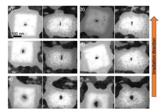
Fig. 5 TEM images of fabricated nanorods with different orientations embedded in 100 nm ALD-SiO $_2$  and irradiated with 50 MeV  $^{127}$ I at  $10^{14}$  ions per cm $^2$  before (left) and after (right) the irradiation. (a) Length = 34.0 nm and diameter = 19.9 nm, (b) length = 32.0 nm and diameter = 22.3 nm, (c) length = 42.6 nm and diameter = 23.4 nm and (d) length = 34.0 nm and diameter = 19.9 nm, (e) length = 50.4 nm and diameter = 31.2 nm, and (f) length = 70.4 nm and diameter = 42.3 nm.
