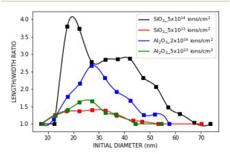
Fig. 10 Comparison of the elongation ratio vs. initial diameter for the nanoparticles embedded in ALD-SiO<sub>2</sub> (ref. 32) and ALD-Al<sub>2</sub>O<sub>3</sub>. The uncertainties are left out from the image for clarity.
